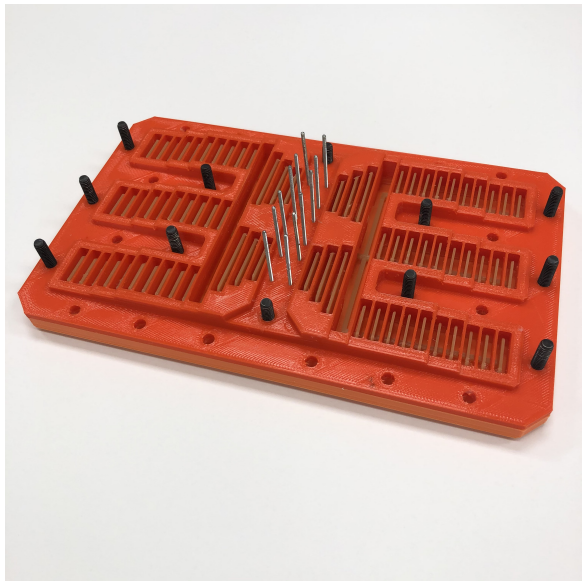
Figure 3.3: Assembled Top Mold
