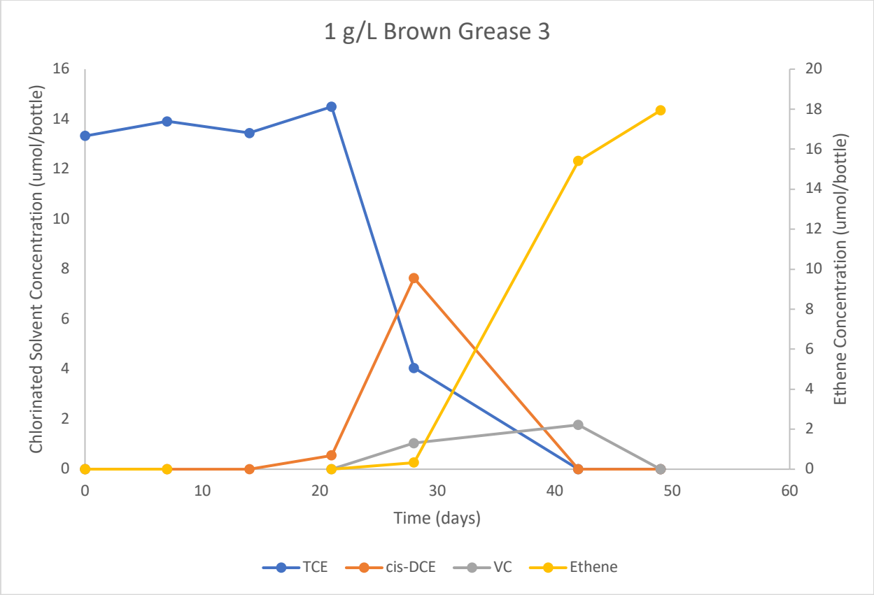
Appendix Figure 9. 1 g/L Brown Grease dosed bottle. Chlorinated solvent concentration over time in feasibility experiment with soil collected from Easley, South Carolina.
