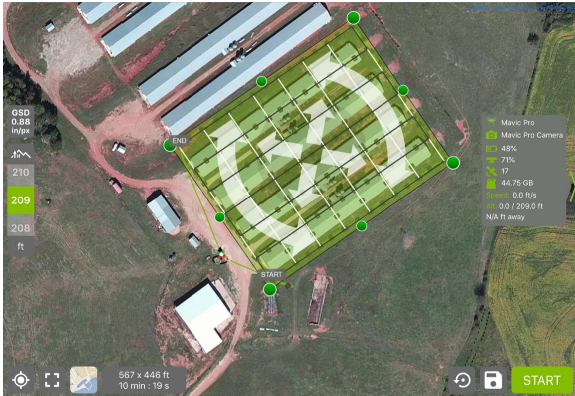
Figure 0.4 Sample image of the UAV flight path in Pix4D Capture (Pix4D, 2017).
