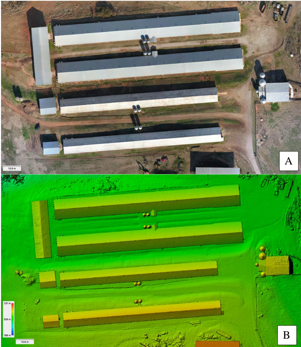
Figure 2.7 (a) Orthomosaic image (14,335x11,647, 1.93 cm/px) and (b) DSM (9,548 x 7,884, 3.86 cm/px) built from Dense Point Cloud (DPC).
