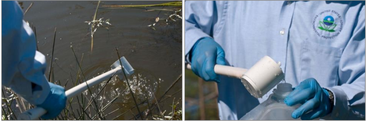
Figure 4.2. Photos demonstrating the use of the long-handled dipper for collecting sample water and filling a sample bottle. Photos taken by Eric Vance, EPA Photographer, and shared from the NWCA Field Operations Manual (EPA 2011).
