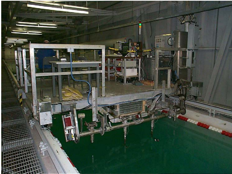
Figure 4. Meter mount on tow cart
