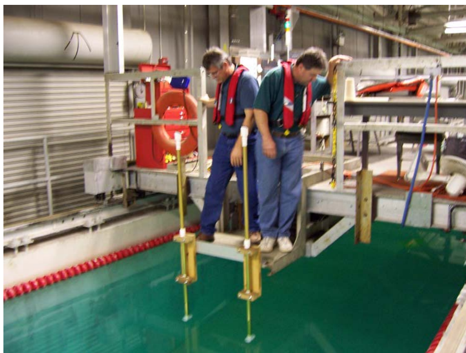
Figure 3. Flow Probe testing in tow tank
