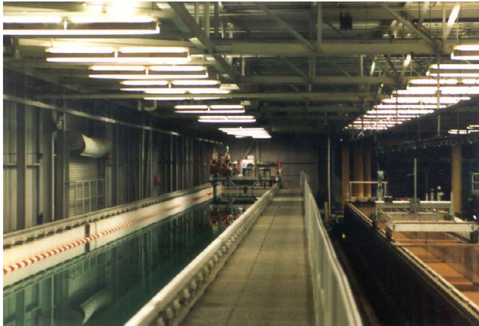
Figure 2. USGS tow tank and tow carriage
