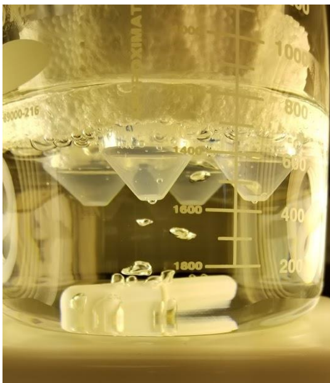
Figure 2.9. Samples being heated at 95 °C and irradiated with UV-B light to form hydroxyl radicals during the peroxide digestion treatment.
