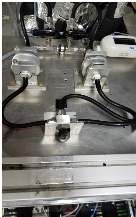
Figure 2.6. The filter collection setup on the NSF/NCAR C-130 for analysis with the IS. Two filters were loaded at any given time, for switching when inside and outside of plumes. Total flow rates were monitored in real-time with the flow meter visible in the upper right.
