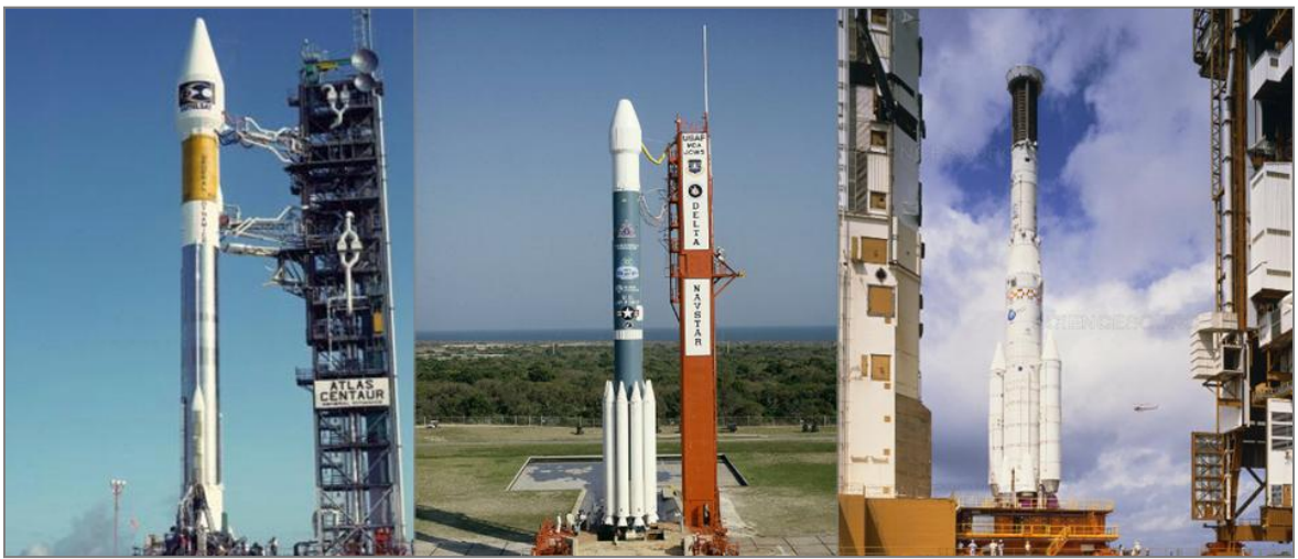
Figure 8-6: Rocket Alternatives A1-Atlas II (left), A2-Delta II (middle), A3-Ariane 4 (right) [123]–[125]
