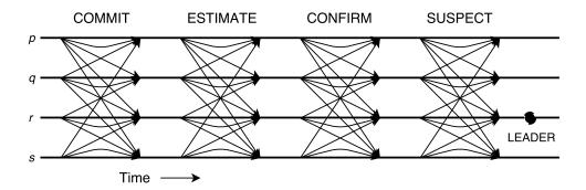
Figure 4.4: Leader Election Protocol Timing Diagram
