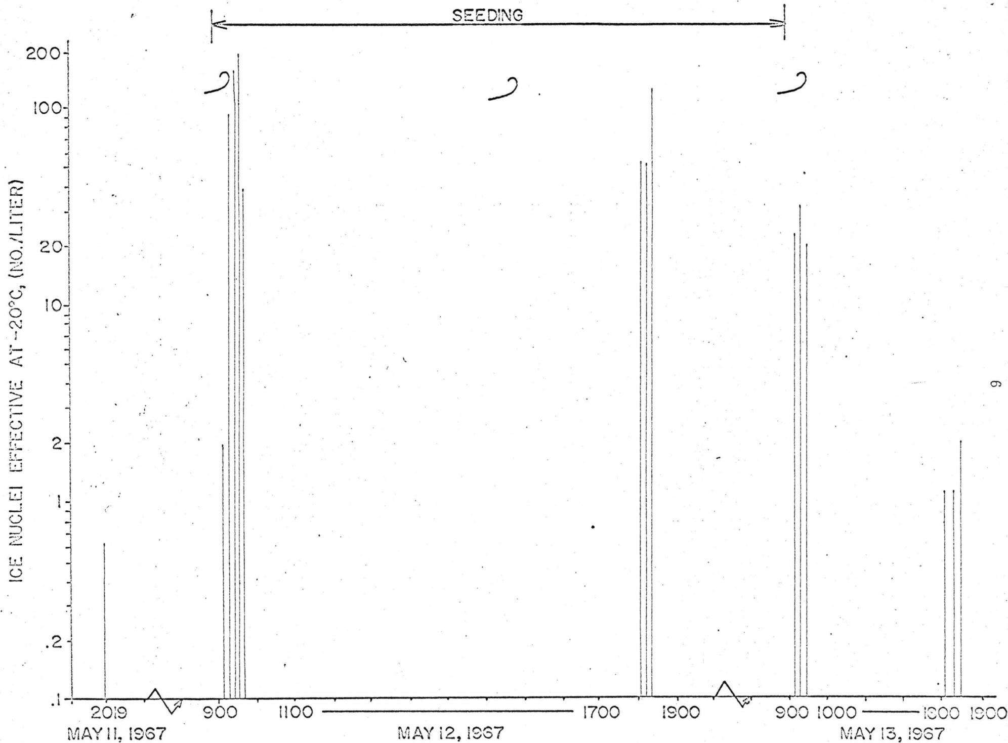
Figure 2. Change in ice nuclei concentrations at Climax after seeding at upwind ground site under clear sunny skies
