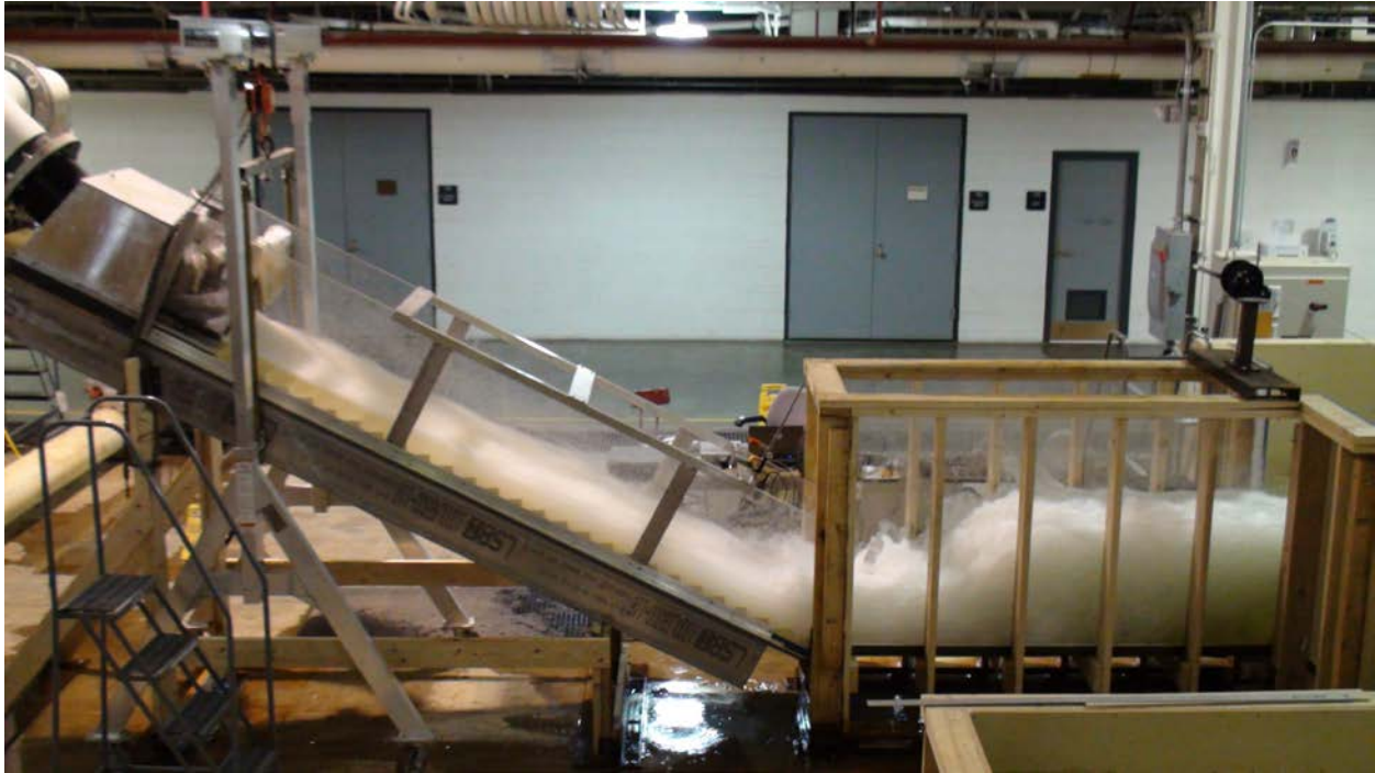
Figure 3. Stilling basin model with stepped chute at 26.57-degrees terminating in a Type III basin
