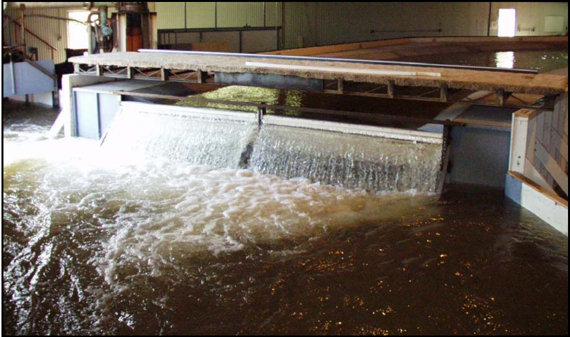
Figure 3.8: Discharge over Stop-log Configuration During Testing
