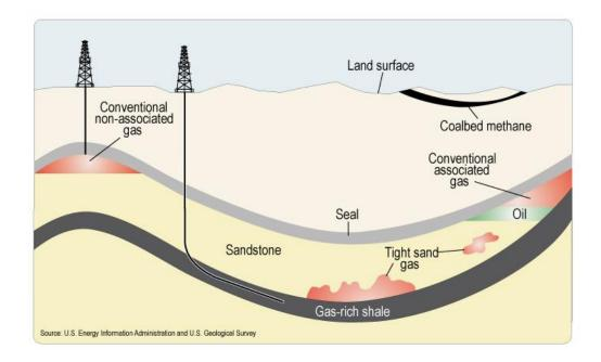
**Figure 1.4**: Cross sectional view of the geology of natural resources underground, including a depiction of horizontal drilling in a gas-rich shale deposit (U.S. Energy Information Administration, 2011).
