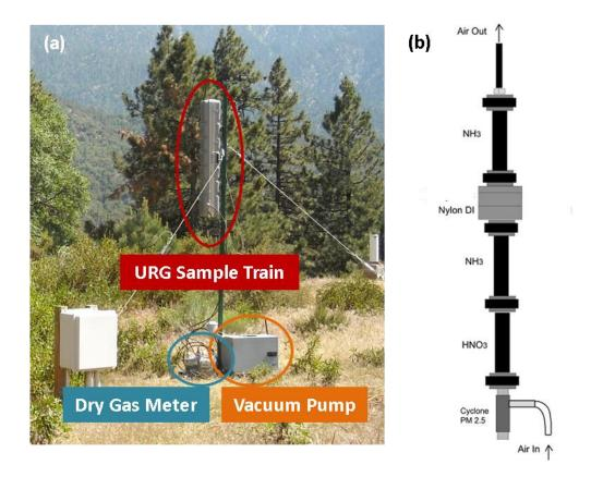
**Figure 2.1**: The URG sampling system set up in the field (a) identifies the vacuum pump, dry gas meter and the protective case for the sampling train. The order of the cyclone, denuders and nylon filter in the URG sample train is represented in (b), which is modified from a diagram in (Yu et al., 2005).
