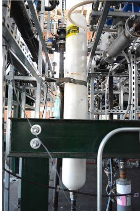
Figure 4-30. Cooling cycle accumulator.
