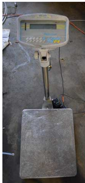
Figure 4-62. Scale used for fill and drain procedures.
