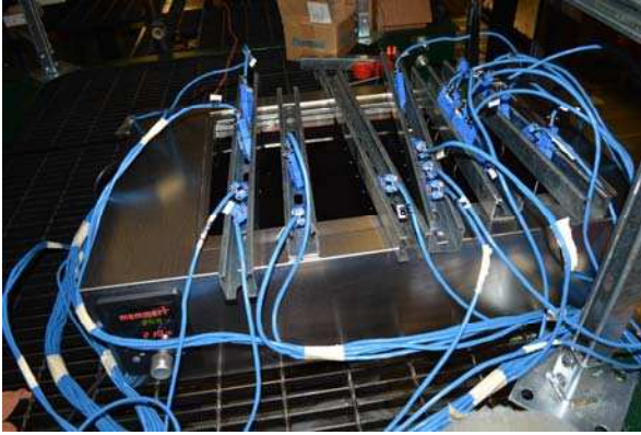
Figure 4-82. Thermocouple oil bath front view.
