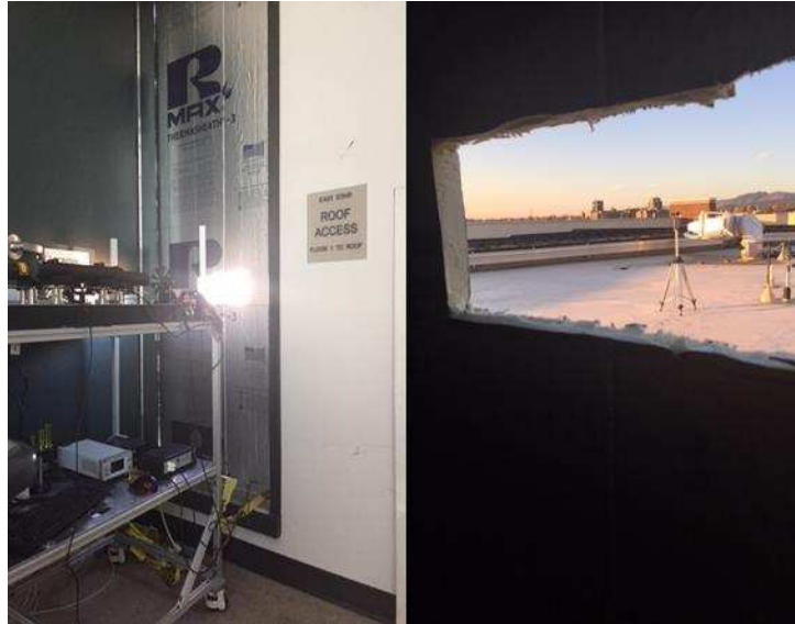
Figure 33: Sensor test location with insulated door (left) and cutout (right) for beam paths.
