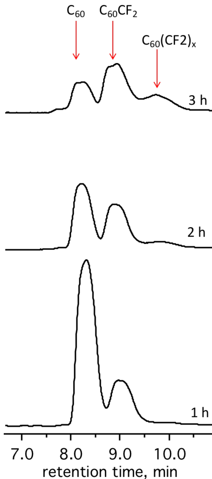
Figure 1.4. HPLC chromatograms of crude C_{60}CF_2 reactions. Increasing reaction time from 1 h to 3 h improves conversion of C_{60} to C_{60}CF_2 . Eluent is toluene at 14 mL/min on a Buckyprep stationary phase measured at 300 nm.
