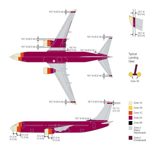
Figure 47. Lightning zone of aircraft
