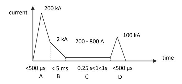
Figure 56. Lightning current waveform as a function of time
