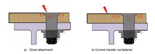
Figure 62. lightning attachment and ignition mechanism
