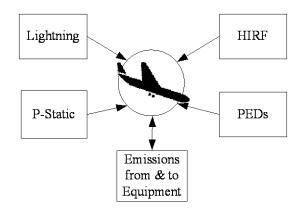
Figure 27. Aircraft electromagnetic effect context diagram
