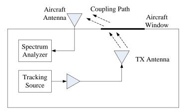
Figure 40. PEDs front door coupling
