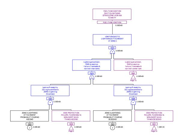
Figure 72. Fault tree for the altitude range from 40,000 to 45,000 ft
