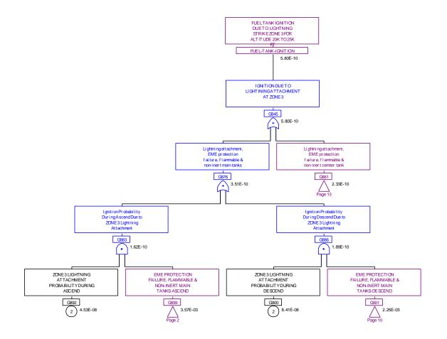
Figure 68. Fault tree for the altitude range from 20,000 to 25,000 ft
