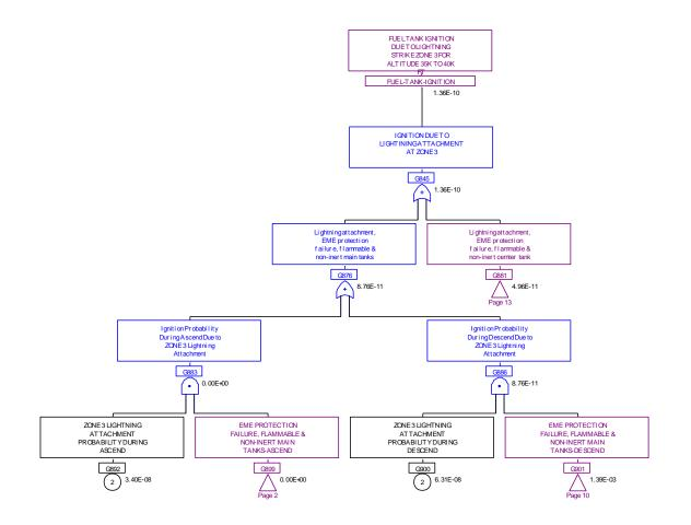
Figure 71. Fault tree for the altitude range from 35,000 to 40,000 ft
