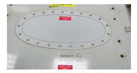
Figure 57. Typical fuel tank door configuration
