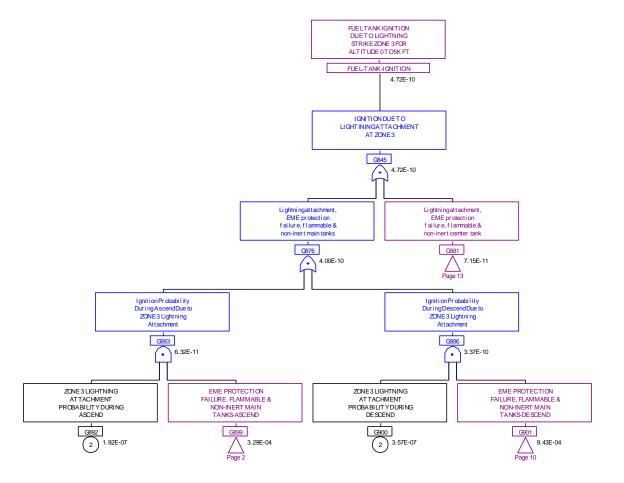
Figure 64. Fault Tree for the altitude range from 0 to 5000 ft
