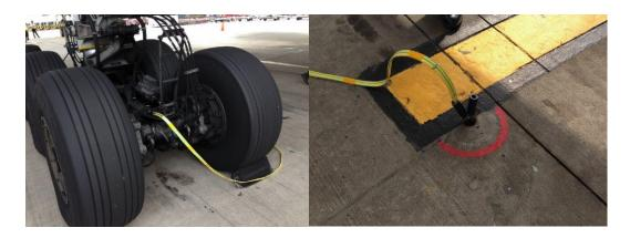
Figure 75. Connection of the grounding cable from the landing gear to ground post in airport Let's use  $0.25 \ge 10^{6} [A^{2} \ s]$  for Zone 2 (component D) where the action integral is  $0.56 \ge 10^{6}$  for the 10 AWG wire with cross section  $0.0526 \ cm^{2}$
