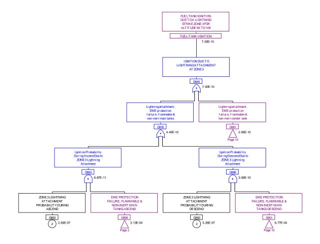
Figure 65. Fault tree for the altitude range from 5,000 to 10,000 ft
