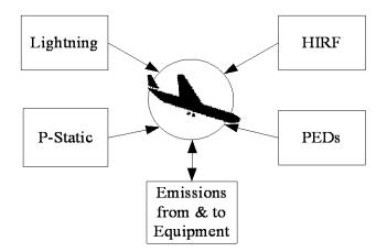
Figure 13. Aircraft electromagnetic context diagram
