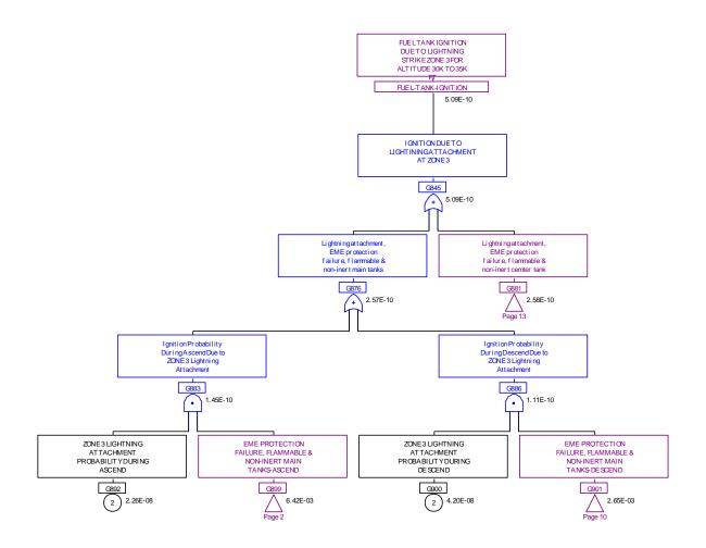
Figure 70. Fault tree for the altitude range from 30,000 to 35,000 ft
