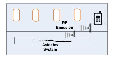
Figure 41. PEDs back door coupling
