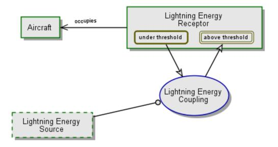
Figure 46. Lightning energy coupling modeling with OPM
