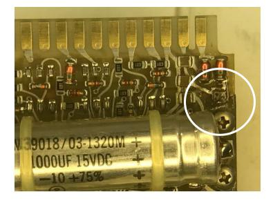
Figure 10. Burnt circuit in lavatory drain control logic represents issues and risk
