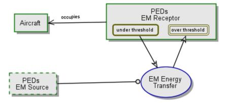
Figure 28. Portable electronic device energy coupling diagram with OPM modeling. PEDs EM sources are part of the environment with dotted lines
