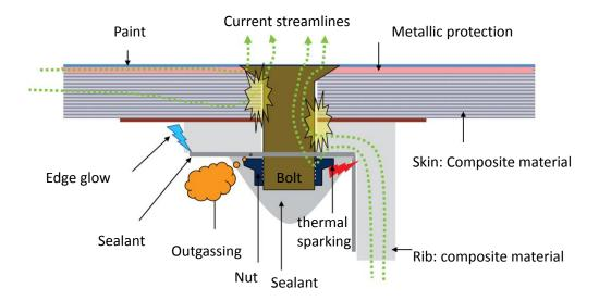
Figure 63. Sparking mechanism due to lightning current
