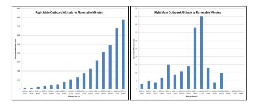
Figure 74. Flammable minutes vs. altitude ranges for right main outboard fuel tank for ascent phase (L) and descent phase (R)
