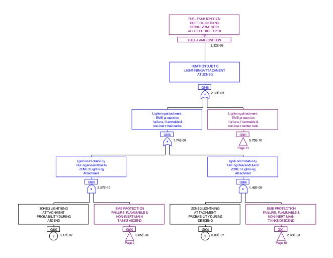
Figure 66. Fault tree for the altitude range from 10,000 to 15,000 ft
