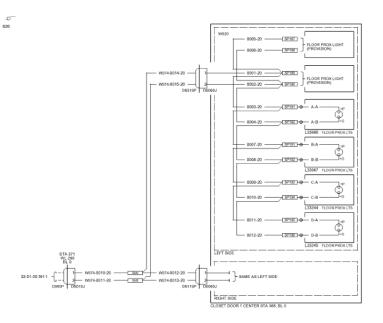
Figure 17. Wiring diagram of emergency floor proximity light system
