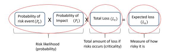
Figure 49. Expected loss calculation diagram
