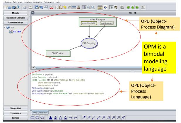
Figure 9. OPCAT suite for EMI energy coupling model
