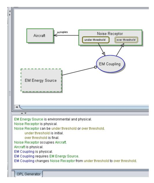
Figure 32. Modeling of EM energy source coupling to receptor with OPM in OPCAT suite
