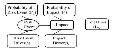
Figure 36. Standard risk model to be used for electromagnetic effects analysis
