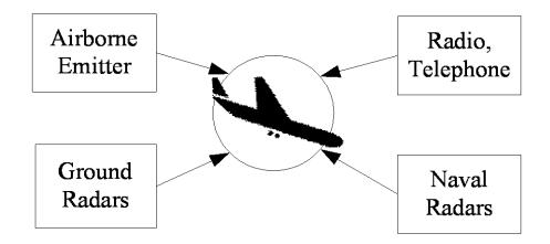
Figure 39. HIRF effect in aircraft context diagram
