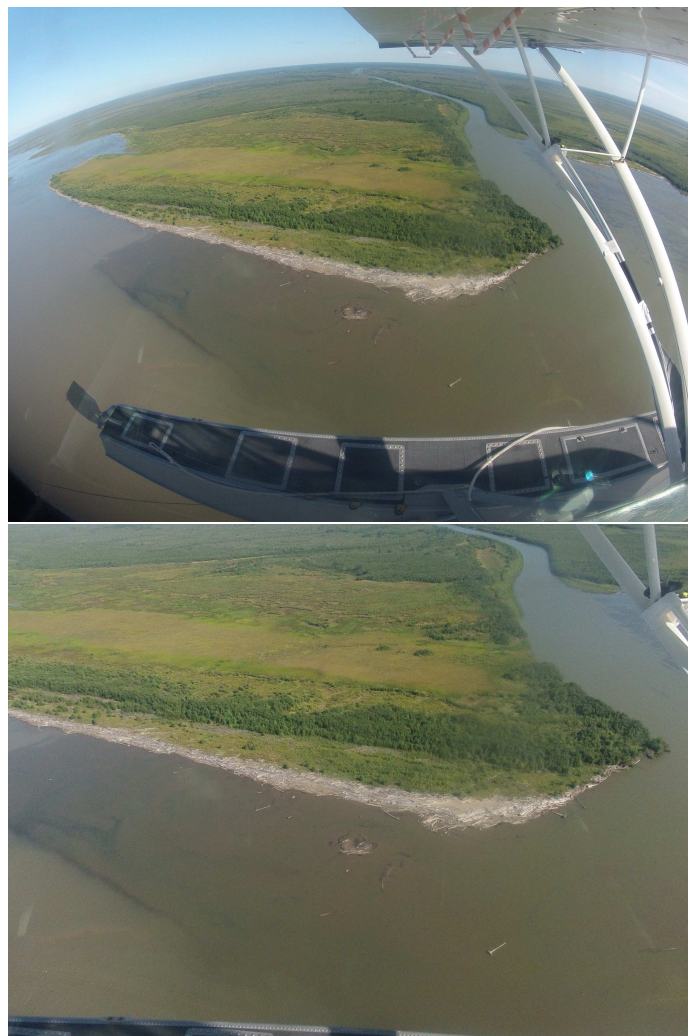
FIGURE 3.C.2. Photo on the left shows the original fish-eye distortion and the photo on the right shows the photo corrected for distortion, cropped and ready for analysis.
