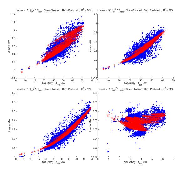
Figure V.21 -  $I^2R$  losses in MW observed and predicted in the system's transmission lines, as a function of  $P_{out}$  in MW
