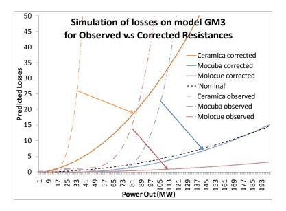
Figure V.24 - Comparison of  $I^2R$  theoretical losses for Ceramica, Mocuba and Molocue substations, calculated before and after correction of the observed losses by the empirical resistance
