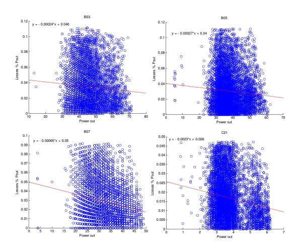
Figure V.30 – Hourly Energy Losses recorded for Transmission lines
