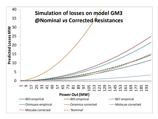
Figure V.34 - Calculation of I<sup>2</sup>R losses using by model GM3
