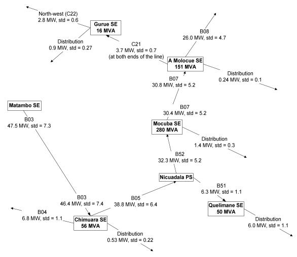
Figure V.26 - Means and standard deviations in the recorded (active) power flows
