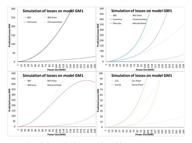
Figure V.33 - Calculation of I<sup>2</sup>R losses using by model GM1
