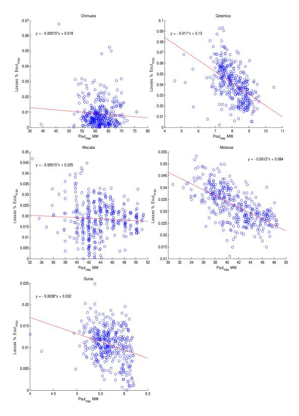
Figure V.29 - Daily Energy Losses recorded for the Substations
