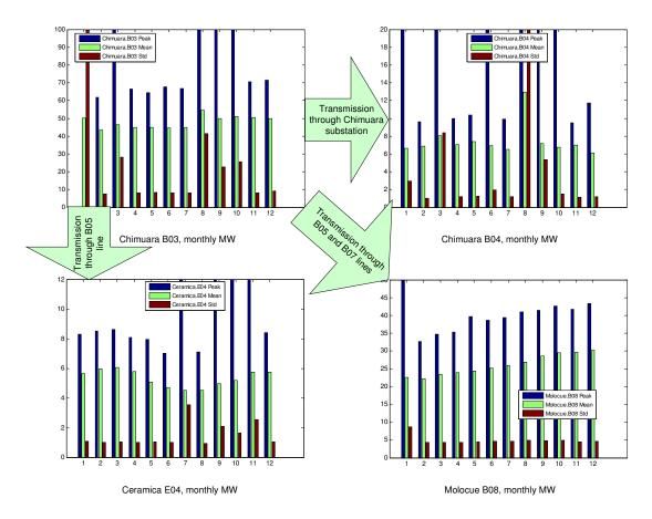
Figure V.27 - Monthly loads at line (B03) and the main load centers
