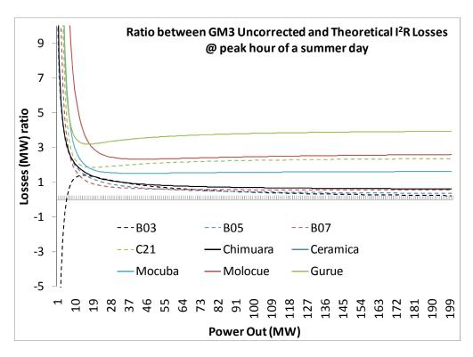
Figure V.35 – Ratio between uncorrected GM3 simulated losses and the theoretical losses
