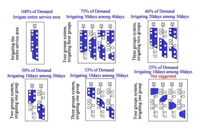
Figure 6. Example of Rotational Irrigation Applied to Lateral Canal System
