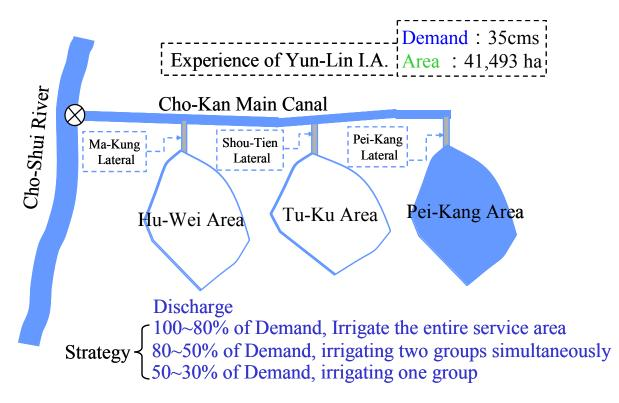
Figure 5. Example of Rotational Irrigation Applied to Main Canal System
