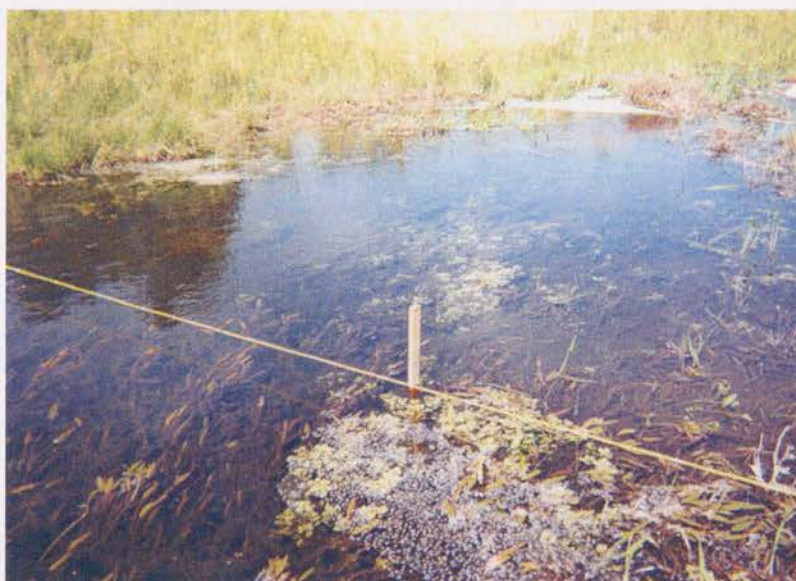
Figure 4.2. Gage 2 and Line for Sectioning Off Cross-Section for Discharge (April 2003).
