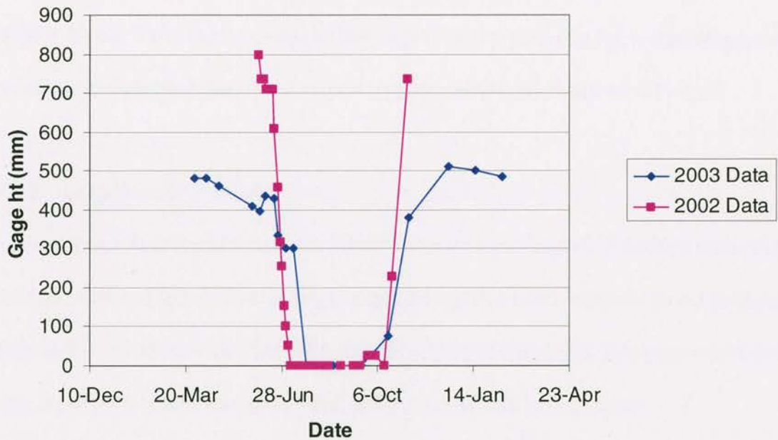
Figure 4.5 (a) and (b). Stage Heights for Gages 1 and 2 (2002 and 2003).
