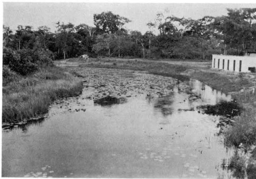
View from the bridge looking at the downstream reach of the Río Mapirito. The discharge was gaged in this reach. Note the vegetation in the channel and on the banks.
