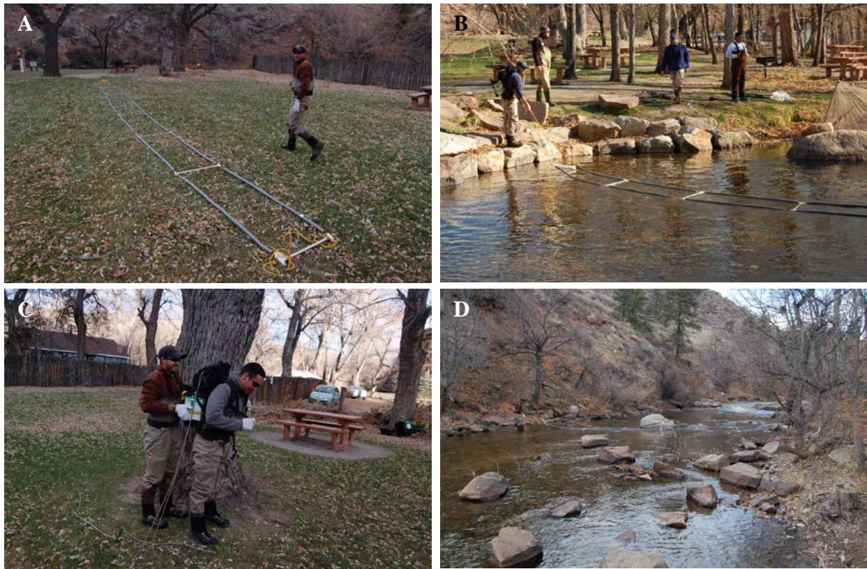
Figure A3.2-2. The shore-deployed floating antenna array, 14.6 x 0.6 m, was constructed using eight gauge speaker wire; PVC supports placed every 1.8 m helped maintain array shape (A). Foam pipe insulation was used to float the array on the river surface and the array was controlled using floating nylon rope (B). The sling-load pack was carried by one operator and housed the 12-V marine, deep-cycle battery, reader, and tuner box (C); a second operator helped maintain array shape and guide the array over obstacles in the river (D).
