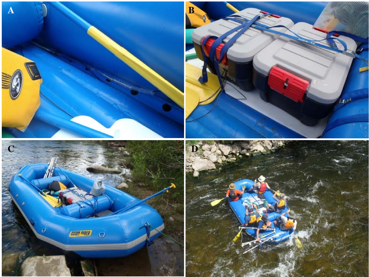
Figure A3.2-1. Twelve gauge THHN wire was used to create the horizontal and vertical arrays of the raft antenna system. For the horizontal array, proximity of the wire and array shape were maintained using flexible plastic tubing secured to the self-bailing holes using soft nylon cord (A). Submersion of electronic equipment was prevented by storing the equipment in top-locking plastic containers strapped to a rigid plastic deck on the bottom of the raft (B). The design of the vertical array allowed it to be stored in accordion-like fashion when not in use (C) and facilitated quick deployment in holes deeper than one meter (D).
