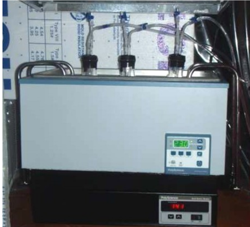
Figure 3: Actual growth system: Temperature and mixing maintained with a shaking water bath, light supplied with a 1000 watt daylight metal halide grow lamp, headspace gas supplied and sampled with tubing, stopcocks, and rubber stoppers.
