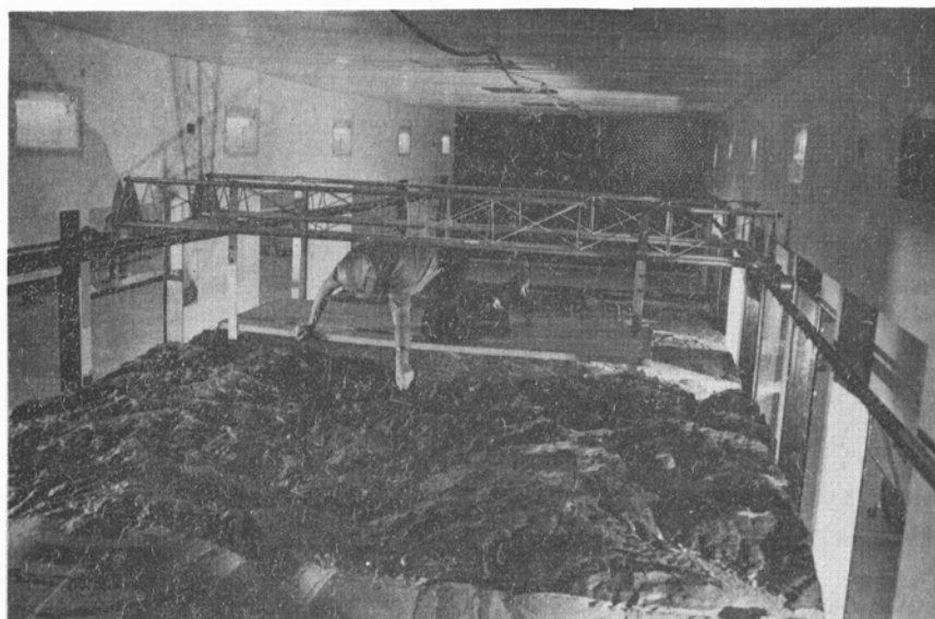
Fig. 12 San Juan topographic model as presently arranged in the Colorado State University environmental wind tunnel.
