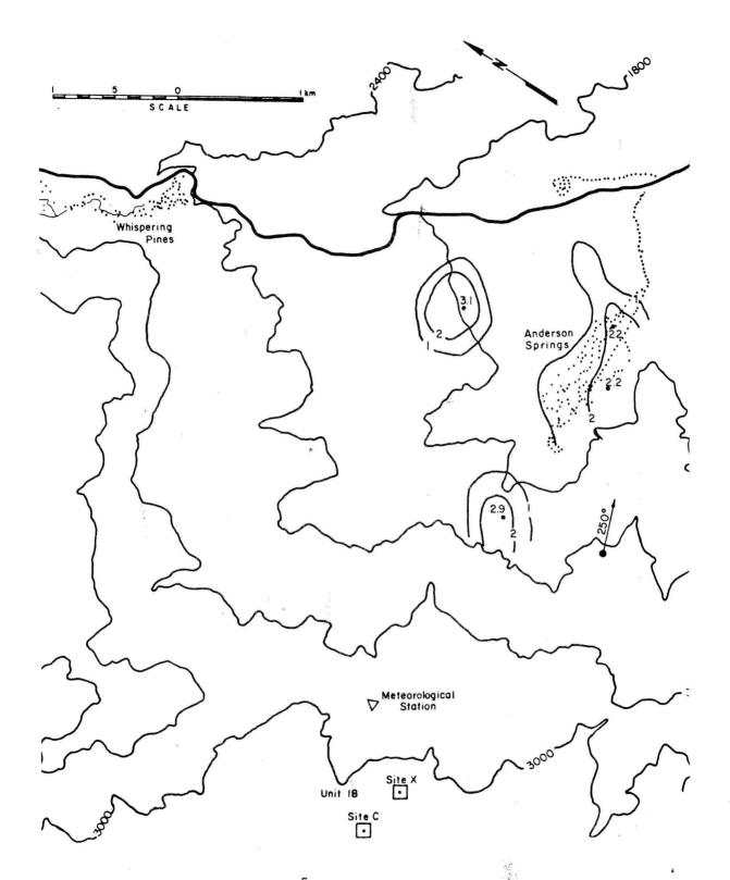
Figure 5.2-3d. Isopleths (x 10<sup>5</sup>) of nondimensional concentration coefficient K for Unit 18, Site C, a 250° wind direction and wind speeds of a) 3.1, b) 4.5, c) 8.9 and d) 11.6 m/s.
