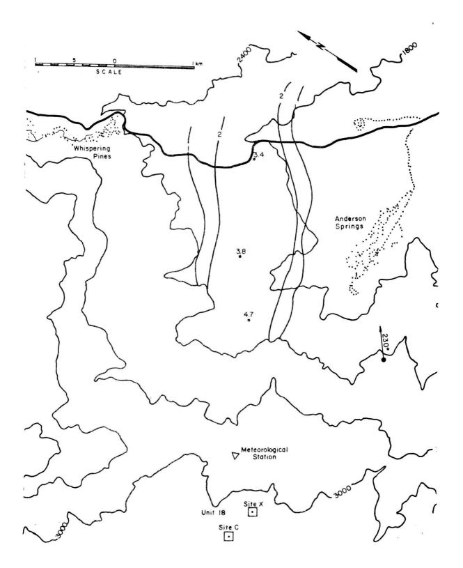
Figure 5.2-2c. Isopleths  $(x \ 10^5)$  of nondimensional concentration coefficient K for Unit 18, Site C, a 230° wind direction and wind speeds of a) 3.1, b) 4.5, <u>c) 8.9</u> and d) 11.6 m/s.
