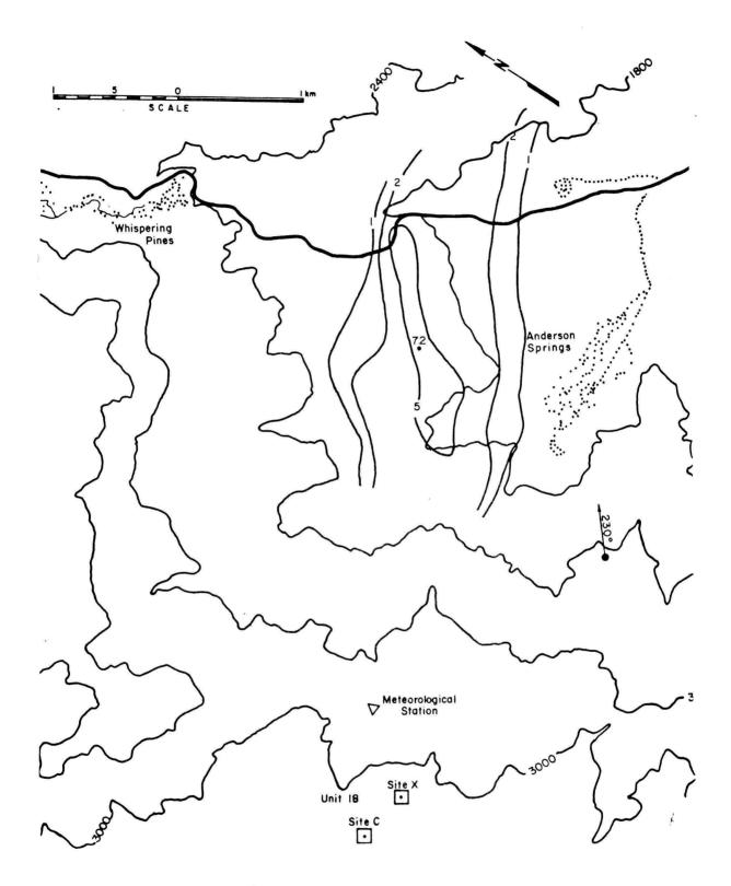
Figure 4.2-2c. Isopleths  $(x \ 10^5)$  of nondimensional concentration coefficient K for Unit 18, Site X, a 230° wind direction and wind speeds of a) 3.1, b) 4.5, <u>c) 8.9</u> and d) 11.6 m/s.
