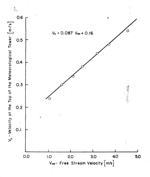
Figure 6-3. Free Stream Velocity Versus the Velocity at the Top of the Meteorological Tower (model) for the 250<sup>°</sup> Wind Direction
