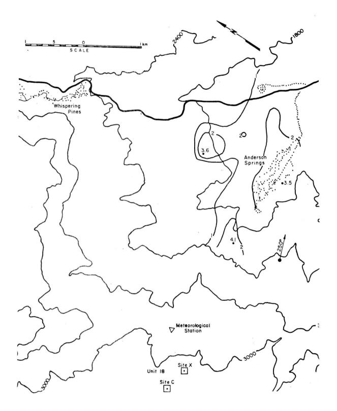
Figure 5.2-3c. Isopleths  $(x \ 10^5)$  of nondimensional concentration coefficient K for Unit 18, Site C, a 250° wind direction and wind speeds of a) 3.1, b) 4.5, <u>c) 8.9</u> and d) 11.6 m/s.
