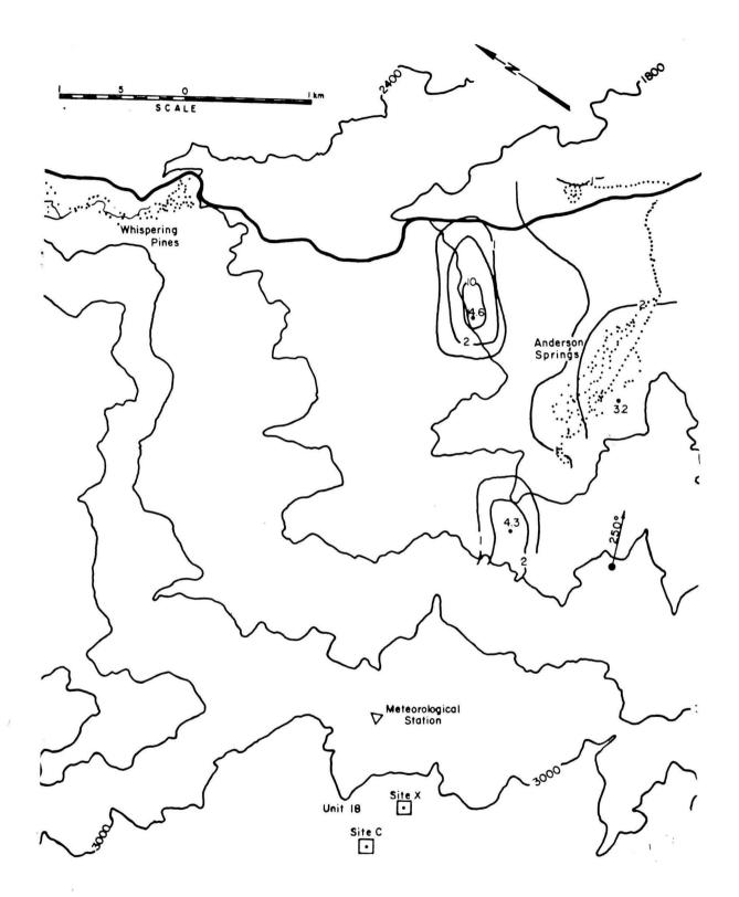
Figure 4.2-3c. Isopleths  $(x \ 10^5)$  of nondimensional concentration coefficient K for Unit 18, Site X, a 250° wind direction and wind speeds of a) 3.1, b) 4.5, c) 8.9 and d) 11.6 m/s.
