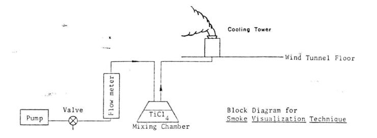
Figure 3.3-1. Schematic of plume visualization equipment.
