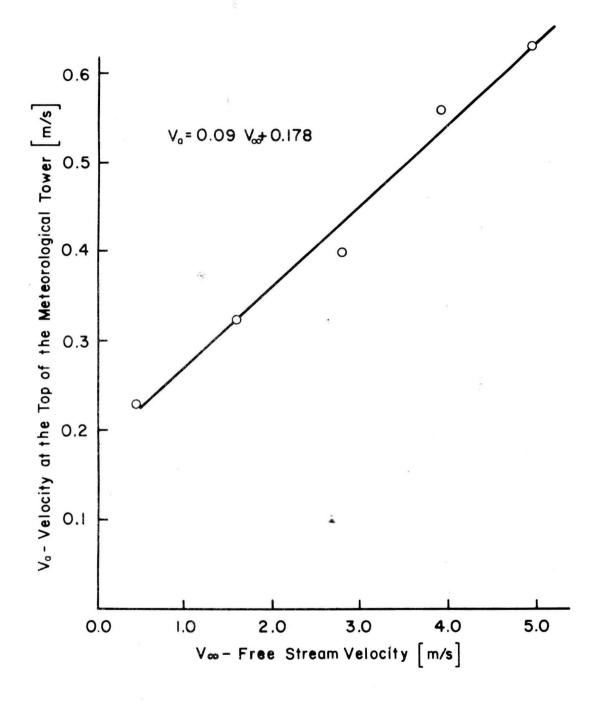
Figure 6-1. Free Stream Velocity Versus the Velocity at the Top of the Meteorological Tower (model) for the 210<sup>°</sup> Wind Direction
