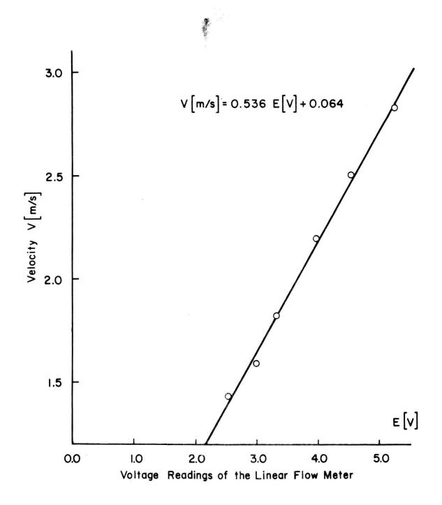
Figure 3.5-1. Calibration Curve for Datametrics Linear Flow Meter
