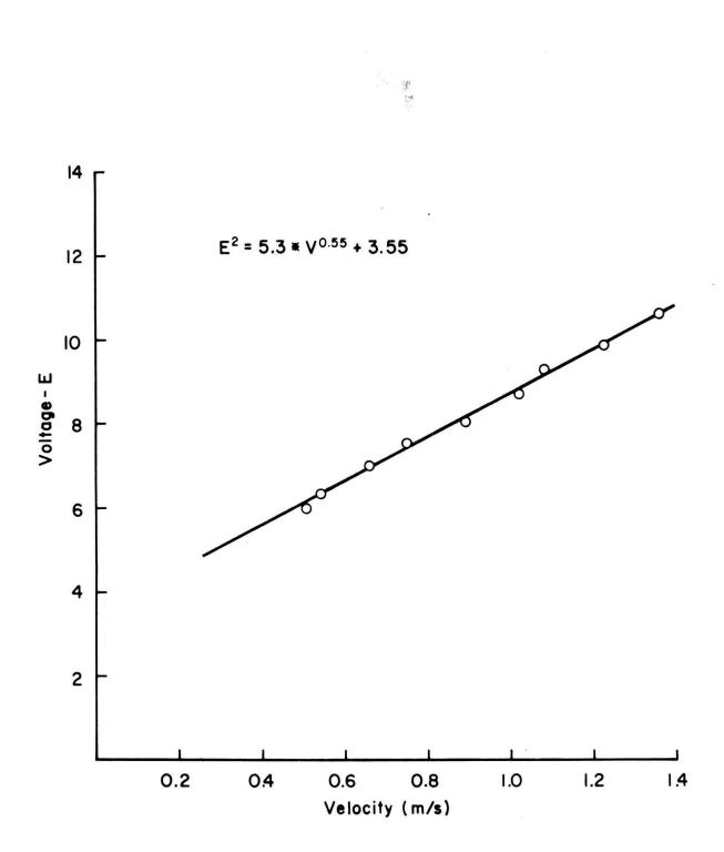
Figure 3.5-2. Calibration Curve for the TSI Hot-Wire Anemometer
