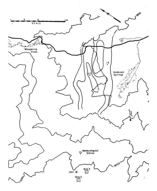
Figure 4.2-2d. Isopleths  $(x \ 10^5)$  of nondimensional concentration coefficient K for Unit 18, Site X, a 230° wind direction and wind speeds of a) 3.1, b) 4.5, c) 8.9 and <u>d) 11.6 m/s</u>.
