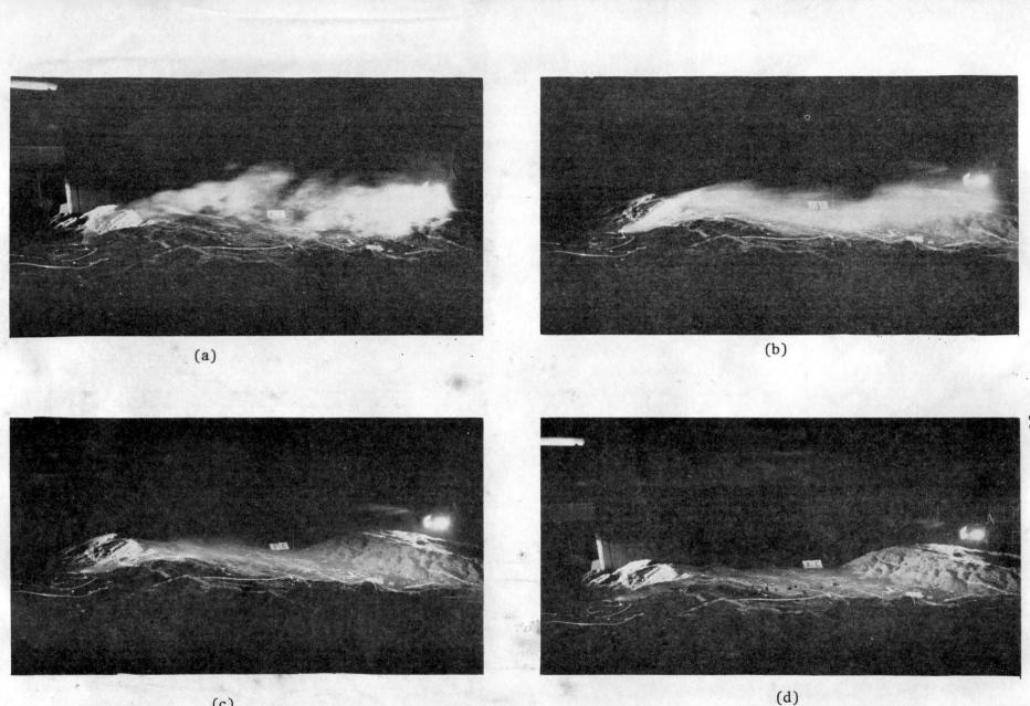
Plume visualizations for Unit 18, Site C, a  $250^{\circ}$  wind direction and wind speeds of a) 3.1, b) 4.5, c) 8.9, and d) 11.6 m/s. Figure 5.1-1.
