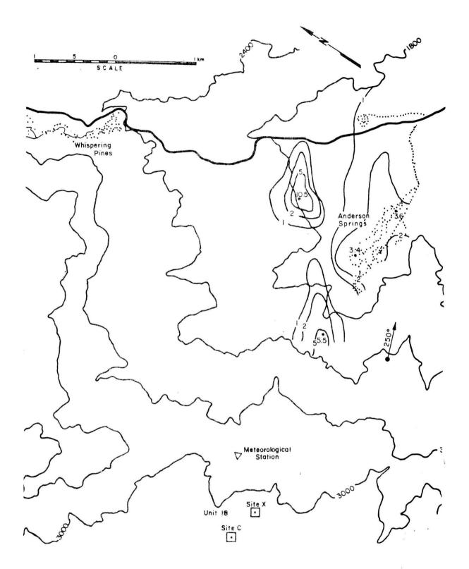
Figure 4.2-3b. Isopleths  $(x \ 10^5)$  of nondimensional concentration coefficient K for Unit 18, Site X, a 250° wind direction and wind speeds of a) 3.1, b) 4.5, c) 8.9 and d) 11.6 m/s.
