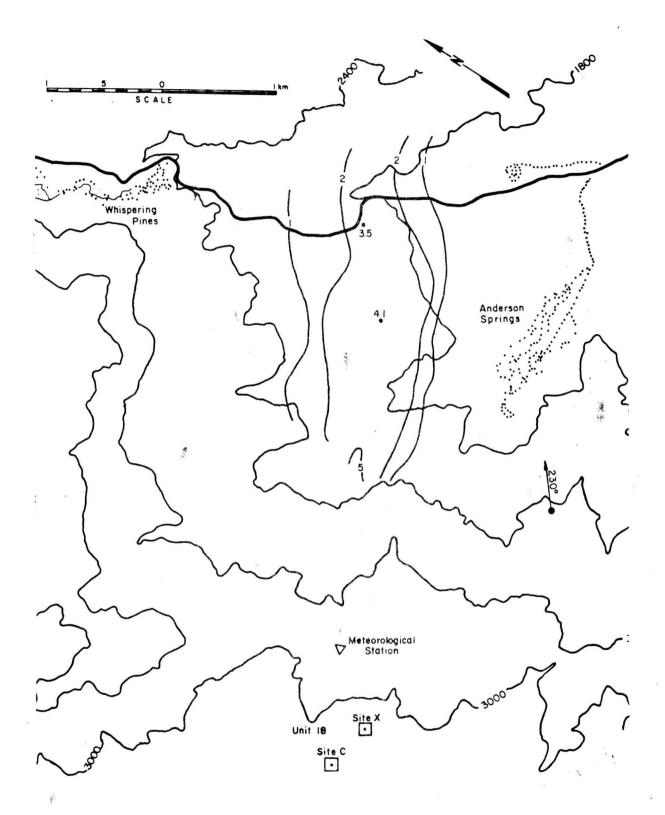
Figure 5.2-2d. Isopleths  $(x \ 10^5)$  of nondimensional concentration coefficient K for Unit 18, Site C, a 230° wind direction and wind speeds of a) 3.1, b) 4.5, c) 8.9 and <u>d) 11.6 m/s</u>.
