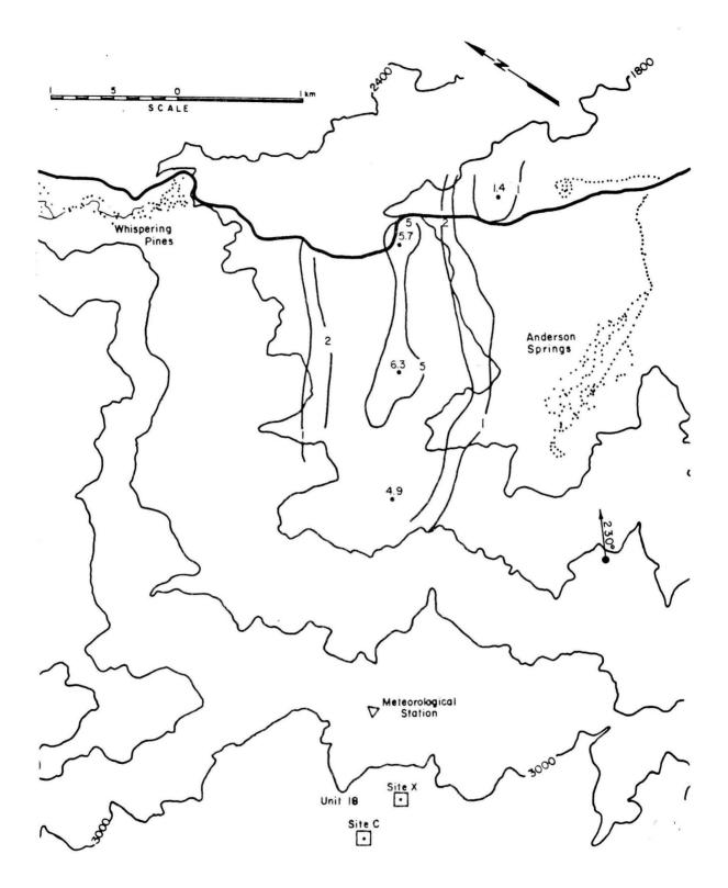
Figure 5.2-2b. Isopleths  $(x \ 10^5)$  of nondimensional concentration coefficient K for Unit 18, Site C, a 230° wind direction and wind speeds of a) 3.1, <u>b)</u> 4.5, c) 8.9 and d) 11.6 m/s.
