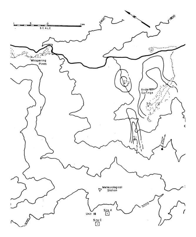
Figure 5.2-3b. Isopleths  $(x \ 10^5)$  of nondimensional concentration coefficient K for Unit 18, Site C, a 250° wind direction and wind speeds of a) 3.1, b) 4.5, c) 8.9 and d) 11.6 m/s.
