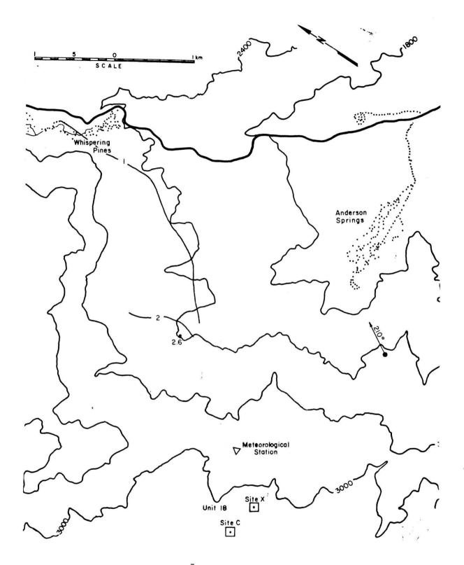
Figure 4.2-1c. Isopleths  $(x \ 10^5)$  of nondimensional concentration coefficient K for Unit 18, Site X, a 210° wind direction and wind speeds of a) 3.1, b) 4.5, <u>c) 8.9</u> and d) 11.6 m/s.
