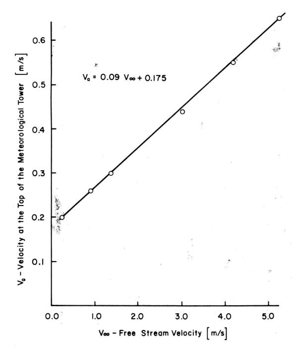
Figure 6-2. Free Stream Velocity Versus the Velocity at the Top of the Meteorological Tower (model) for the 230° Wind Direction
