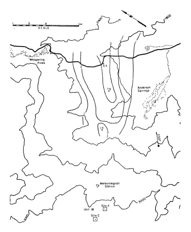
Figure 4.2-2b. Isopleths  $(x \ 10^5)$  of nondimensional concentration coefficient K for Unit 18, Site X, a 230° wind direction and wind speeds of a) 3.1, b) 4.5, c) 8.9 and d) 11.6 m/s.
