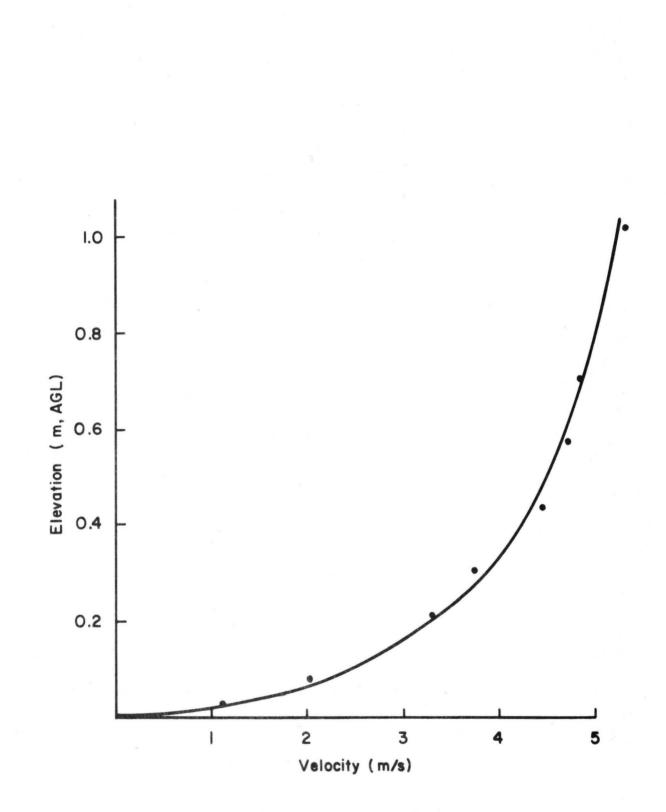
Figure 6-5. Velocity Profile above Site C for the 250° Wind Direction (site elevation--830 m, MSL)
