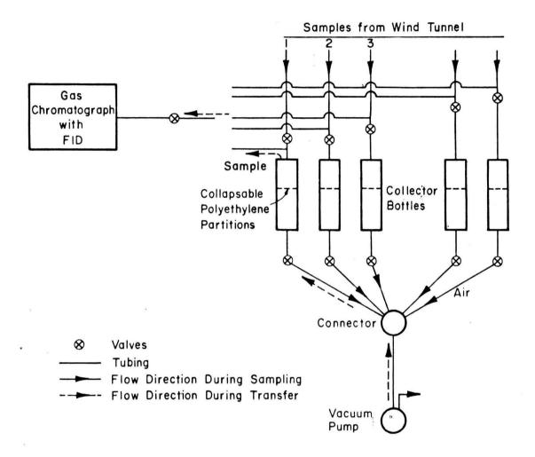
Figure 3.4-1. Schematic of tracer gas sampling system.
