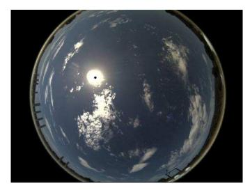
Figure 2-10: Sample image with white cloud edges due to refraction
