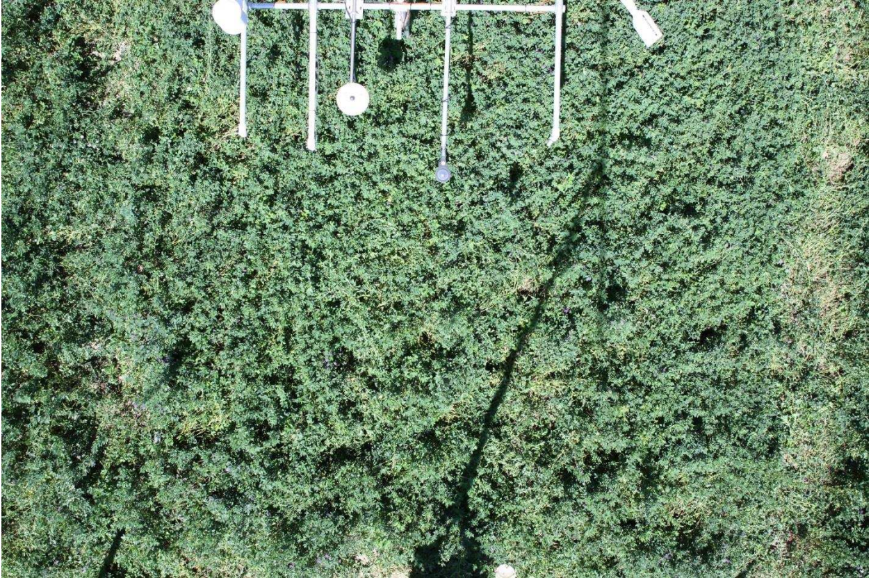
Figure A3: Nadir photo of the lysimeter surface taken on 8/18/2010 ( h_c = 0.52 m, CC = 80.8\% ) (Picture courtesy: Dr. Allan Andales and Lane Simmons)
