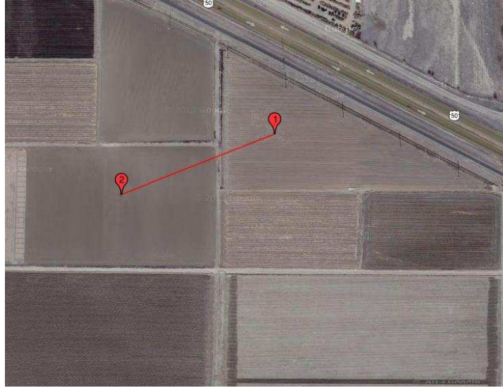
Figure 3.1: Lysimeter fields layout, point 1 showing the reference lysimeter box with triangular field and point 2 showing the crop lysimeter box with rectangular field.
