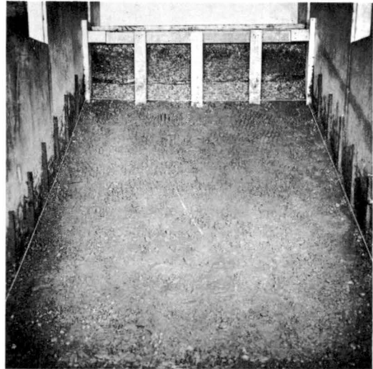
Fig. 18 Unprotected sandy loam backfill before test.
