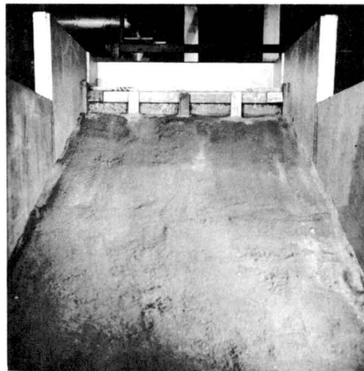
Fig. 11 Unprotected sand backfill before test.
