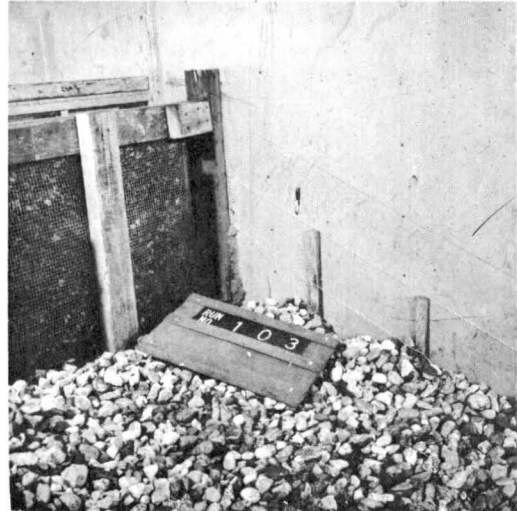
Fig. 14 Result after 12-hour test with 4-inch cover of 1-1/2-inch crushed gravel. Slump at top of test fill was result of soil loss at toe.
