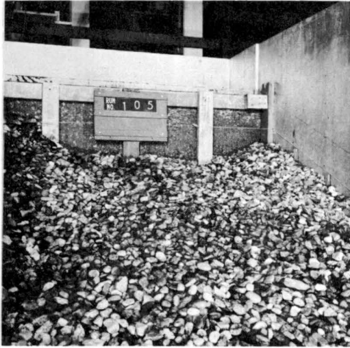
Fig. 16 Result after 12-hour test with 9-inch cover of 1-1/2-inch crushed gravel. Note reduction in slump due to reduction in soil loss through gravel cover.
