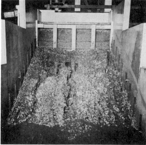
Fig. 19 Result during test of unprotected backfill, 5 minutes after beginning of test.
