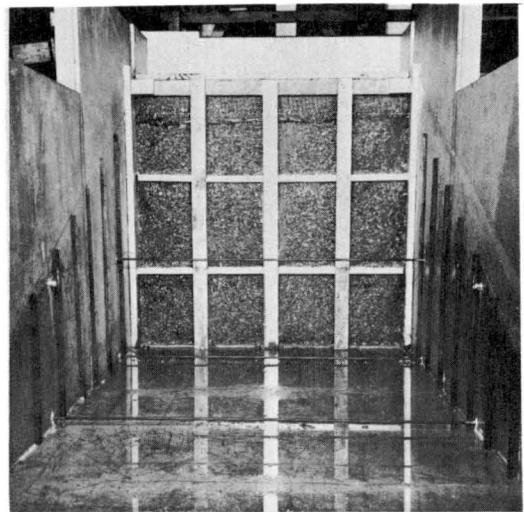
Fig. 6 Inside the box containing the test fill section.
