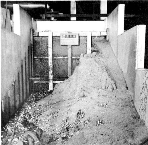
Fig. 12 Result after two-hour test with unprotected sand backfill.
