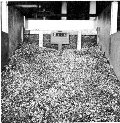
Fig. 13 Result after 12-hour test with 3-inch cover of 3/4-inch crushed rock.
