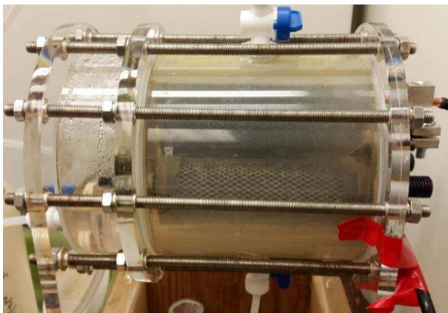
Figure 16 Commercial reactor with cathode mesh visible; anode is within the mesh. Feed chamber at left, vent on top, outlet on the bottom.
