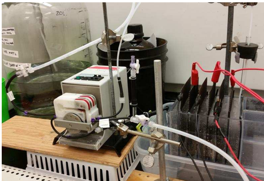
Figure 3 Set-up for bench-scale continuous flow (flow-through) experiments. Feed vessel in left rear, peristaltic pump in center, reactor at right.
