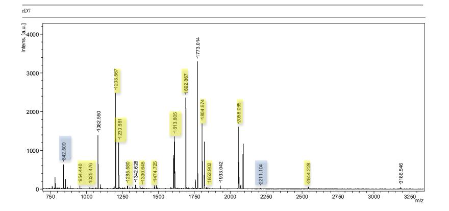
Figure 2.12 Mass spectral analysis of rD7 protein purified from SINV-Ct 3' D7 infected C6/36 cells. Peptide masses are noted above each of the major peaks. These were matched by hand to a theoretical digest of the rD7 protein with trypsin. Yellow highlighted peaks matched to rD7 peptides. Blue highlighted peaks match to trypsin autocleavage peptides and are not associated with rD7.
