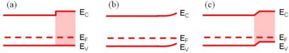
Figure 2.3: Schematics of mechanisms to create an electron reflector: (a) expanded-band-gap layer, (b) reversed back barrier, and (c) heavily-doped back surface. Figure from Ref. [26].
