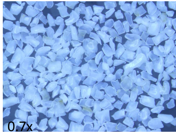
Figure 8: Teeth following crushing and sieving. Teeth are generally uniform in size and no foreign material can be seen (with the exception of stained enamel).
