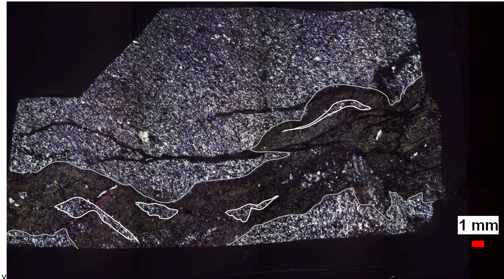
Figure 16. Photomosaic of photomicrographs taken from a thin section of a tourmaline vein express the nature of the quartz lenses included within the tourmaline. Quartz lenses are observed in the middle of the tourmaline vein and are folded with the vein. Because of this, we interpret they formed as a result of a later pulse of meteoric fluid (supported by isotopic data)
