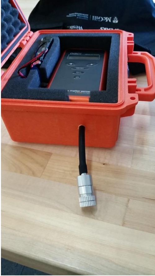
Figure 4.1: Left: DiSCMini instrument used to collect ultrafine particle number concentration. Right: Example set-up of DiSCMini and pDR monitors.
