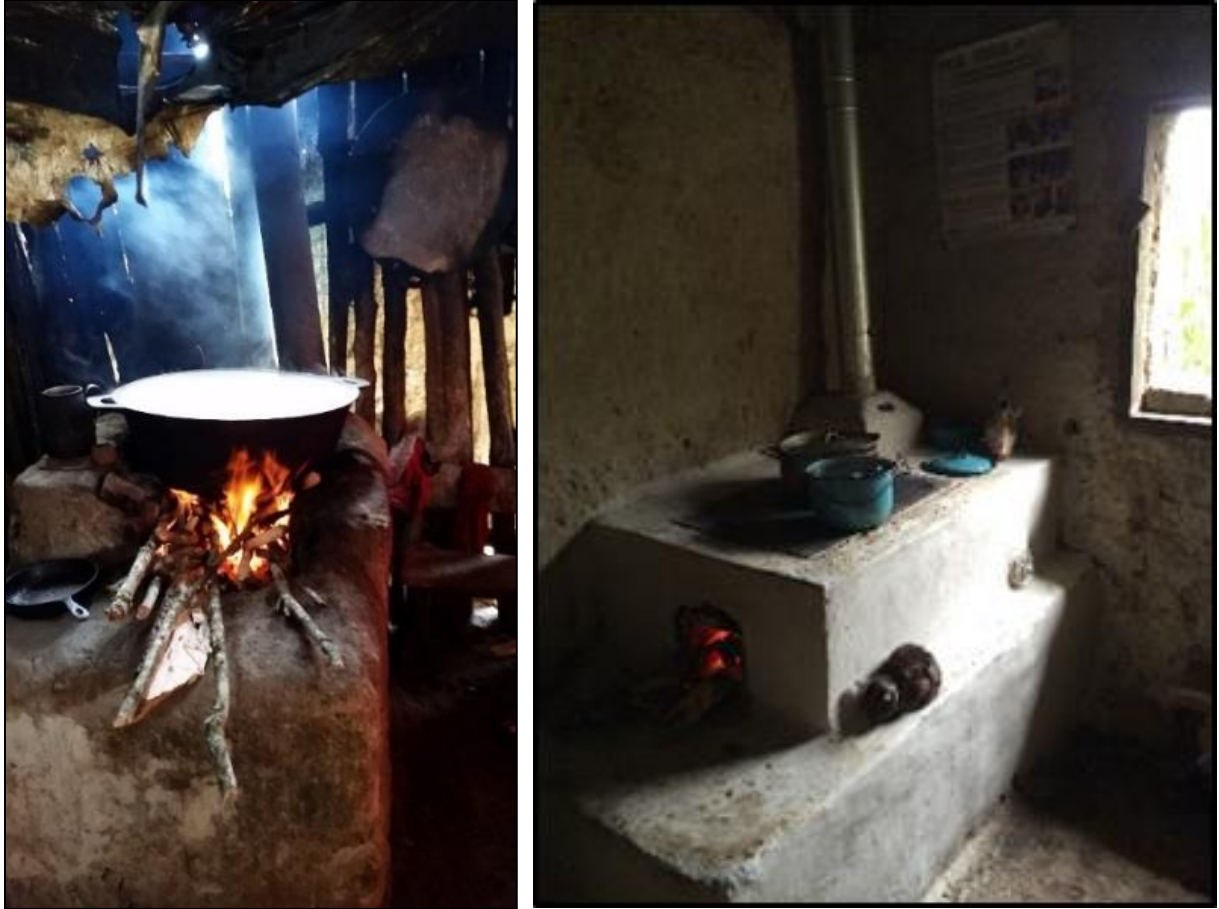
Figure 3.1: Typical traditional (left) and Justa (right) cookstoves in the homes of Honduran women
