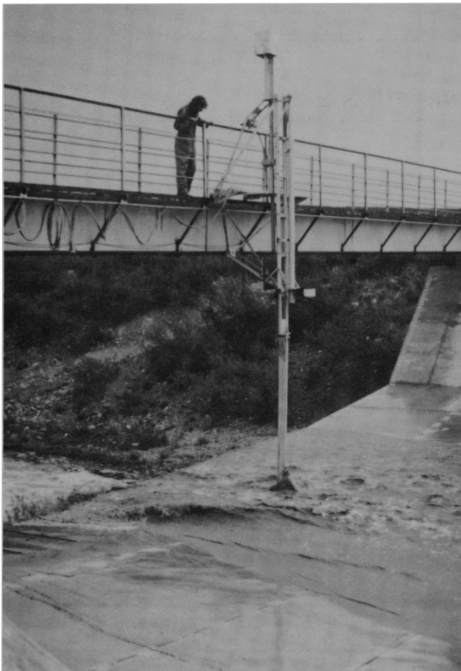
FIGURE 21.—Instrument carriage and velocity meter probe in use at flume 63.006, August 10, 1976. BN-48656
