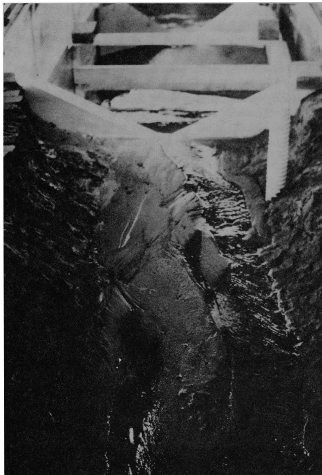
FIGURE 2.—Photograph looking downstream at 1:5 model of Weir 63.113 at Walnut Gulch, after large simulated flow event. The weir exercises no control for lower flows as a result of alluvial filling. BN-48649
