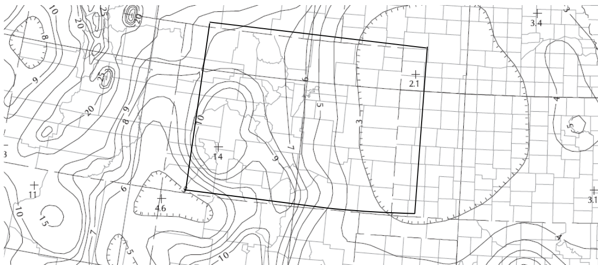
Figure 2.1 Seismic Hazard Maps for AASHTO Guide Specifications, Peak Horizontal Acceleration (7% in 75-year) (2009)
