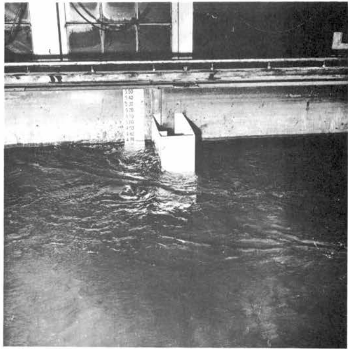
Photo 7 - Model Installed for Scour Test
