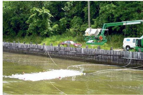
Fig. 1. Photograph of experimental setup at the Naval Research Laboratory's Chesapeake Bay Detachment showing the foam generator floating on the sea surface and the two radiometers in the cradle of a telescopic arm lift.
