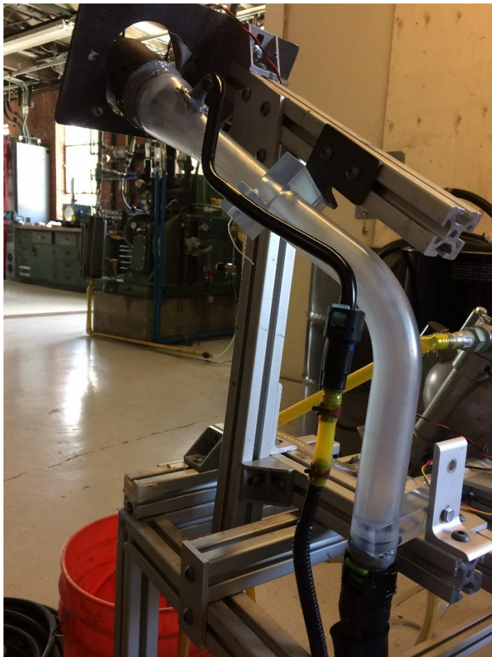
Figure 11: Translucent filler pipe used for high-speed imaging of Stoddard solvent flow in Phase I.
