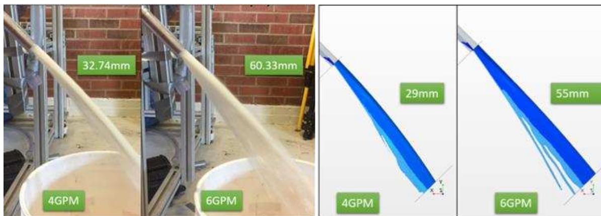
Figure 3: Comparison of experimental and simulated spray widths from Dake et al. for the OPW 11B nozzle at 4 and 6 GPM.
