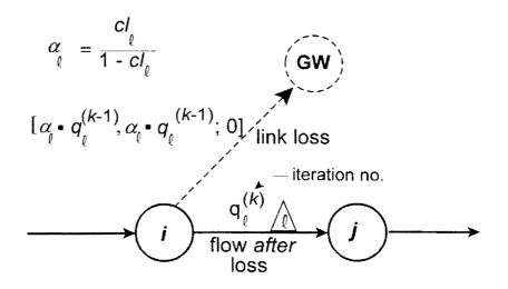
Figure 2.3. Iterative Procedure for Link Loss Calculations
