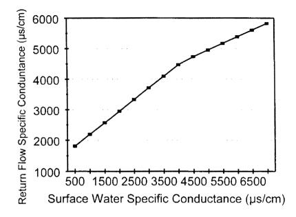
Figure 6.19. Calibration Results of Return Flow Salinity with Groundwater Salinity Set at 4000  $\mu$ S
