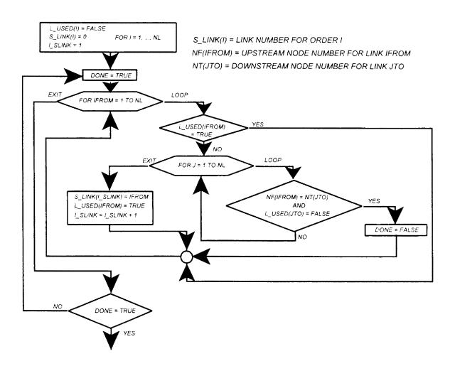
Figure 3.7. Flow Chart for Proposed Numbering Algorithm
