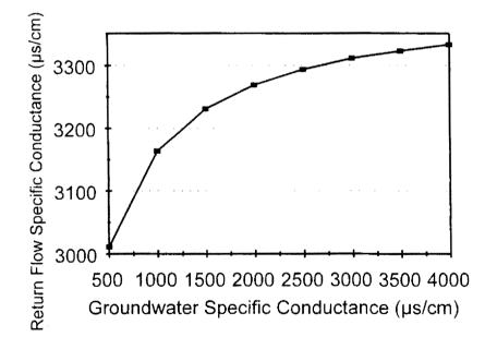
Figure 6.20. Calibration Results of Return Flow Salinity with Surface Water Salinity Set at 2500 µS
