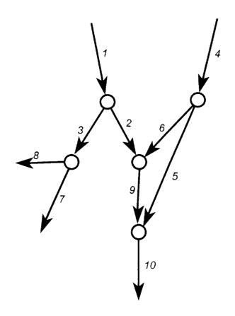
Figure 3.6. Example of the Proposed Stream Reach Numbering Scheme
