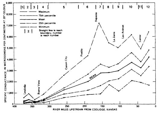
Figure 6.11. Downstream Increase in Specific Conductance of Groundwater in Alluvial Aquifers along the Arkansas River (Cain, 1987)
