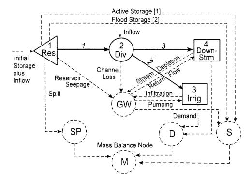
Figure 2.1. Illustration of MODSIM Network Structure with *Accounting* Nodes and Links
