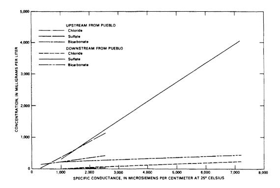
Figure 6.9. Relations of Specific Conductance to Major-Ion Concentrations for Groundwater in Alluvial Aquifers along the Arkansas River (Cain, 1987)
