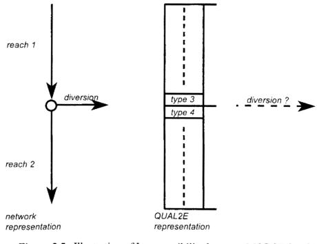
Figure 3.5. Illustration of Incompatibility between MODSIM and QUAL2E
