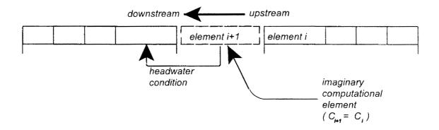
Figure 3.9. Graphical Representation of Modified Approach to Calculating Concentrations
