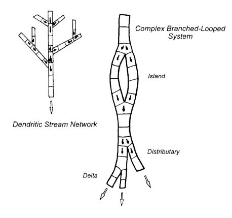
Figure 3.2. Examples of Branched and Dendritic Networks in Onedimensional Models (McCutcheon, 1989).
