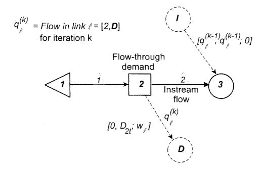
Figure 2.2. Illustration of Flow-Through Demand for Instream Flow Uses
