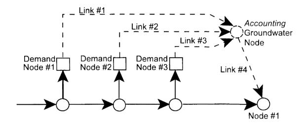
Figure 4.2. River System Network with Return Flows to Accounting Groundwater Node
