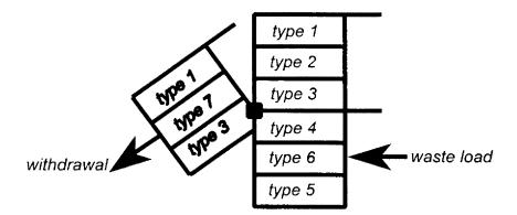
**Figure 3.4**. Illustration of Seven Computational Element Types in QUAL2E (Brown and Barnwell, 1987)
