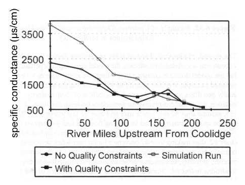
Figure 6.31. Water Quality Results Showing the Effects of Improved Irrigation Efficiency
