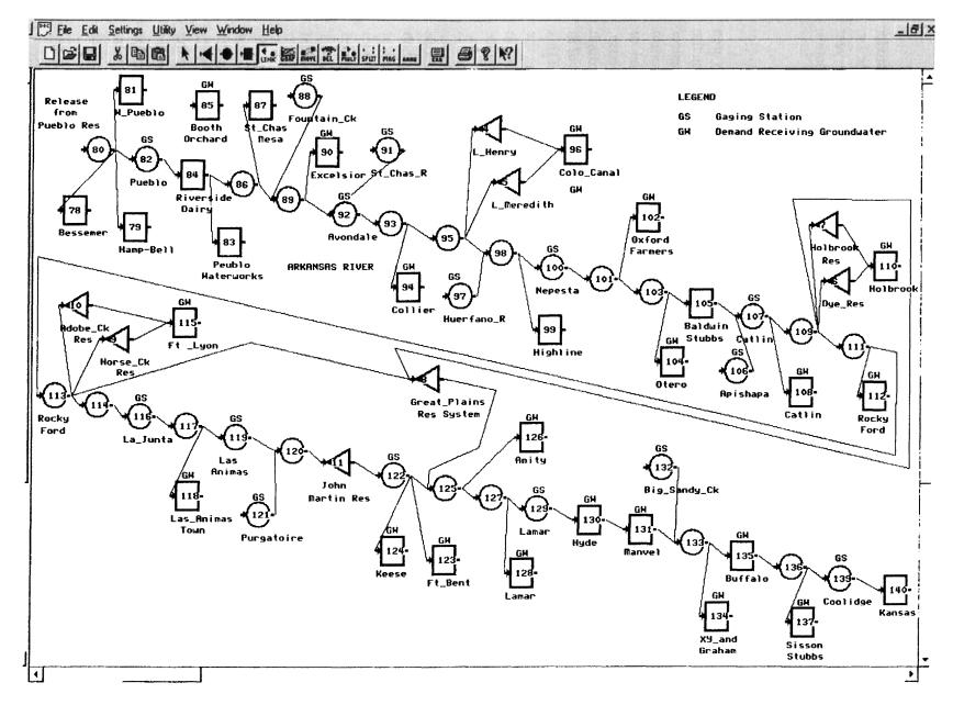
Figure 6.3. Lower Arkansas River Basin Network Configuration in Graphical User Interface for MODSIMQ
