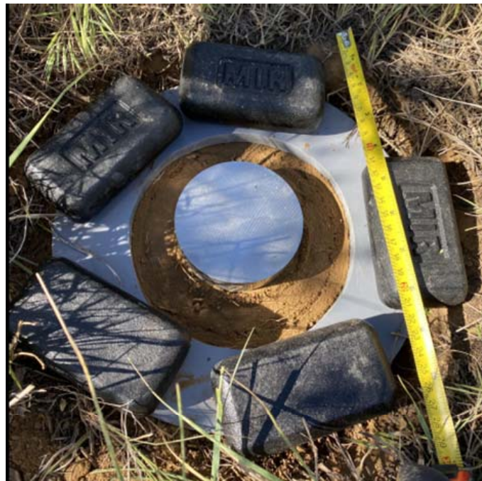
Figure 3.7. Placement of internal and external surcharge on cleared soil surface.
