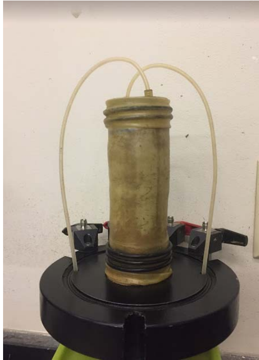
Figure B.6. Soil sample in latex membrane with O-rings placed around the end platens on either end of the specimen to prevent leakage of water into or out of the specimen.
