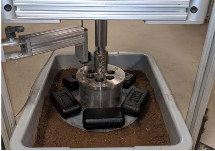
Figure 2.20. Shear annulus placed on a CH in plastic bin with an internal and external surcharge of 2 kPa.
