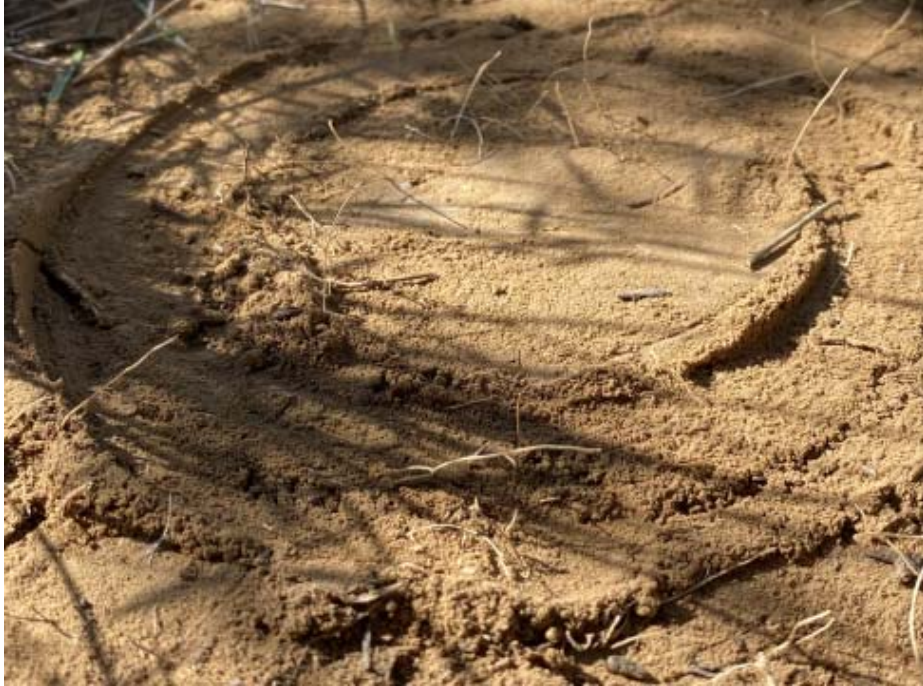
Figure 3.11. Soil surface after shearing by bevameter.
