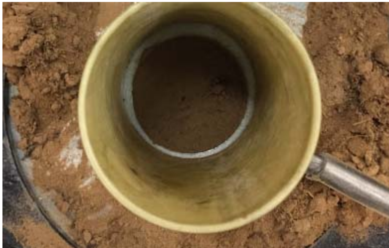
Figure B.5. Latex membrane placed around the sample preparation mold after removal of top 6 mm of soil just before sample is extruded into the membrane.
