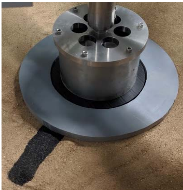
Figure 2.17. Placement of shear annulus and external surcharge ring on SM for shear zone testing.
