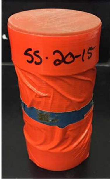
Figure B.4. Sample collected from Drake Farm sealed in a brass sampling tube to preserve in-situ moisture conditions.
