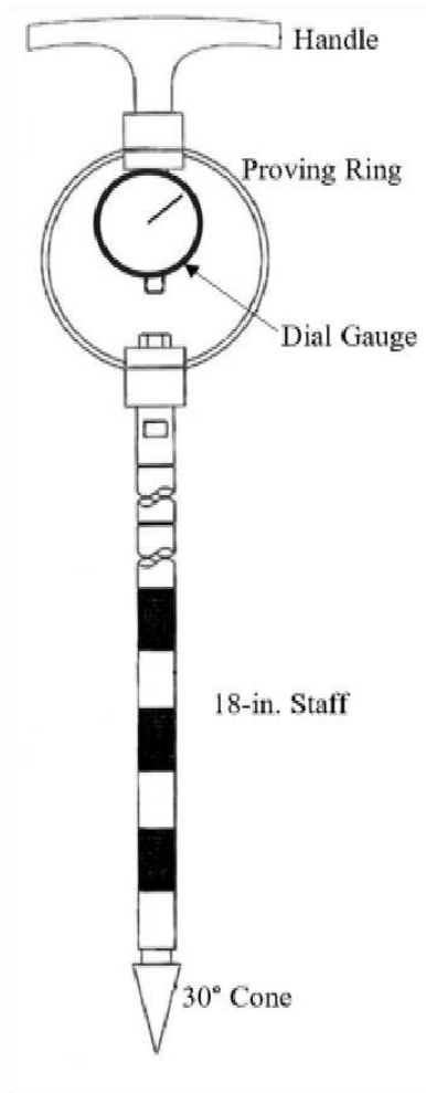
Figure 2.9. Humboldt Manufacturing Co. Corps of Engineers Cone Penetrometer (Humboldt, 2011).
