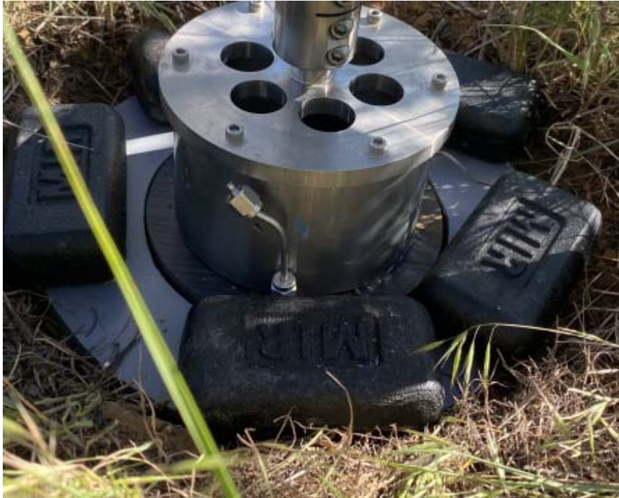
Figure 3.8. Placement of shear annulus on the soil surface with internal and external surcharge.
