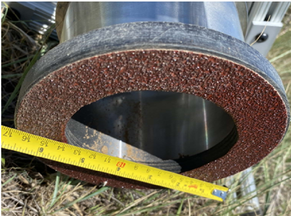
Figure 3.9. Sandpaper as the shear interface on the bottom of shear annulus.
