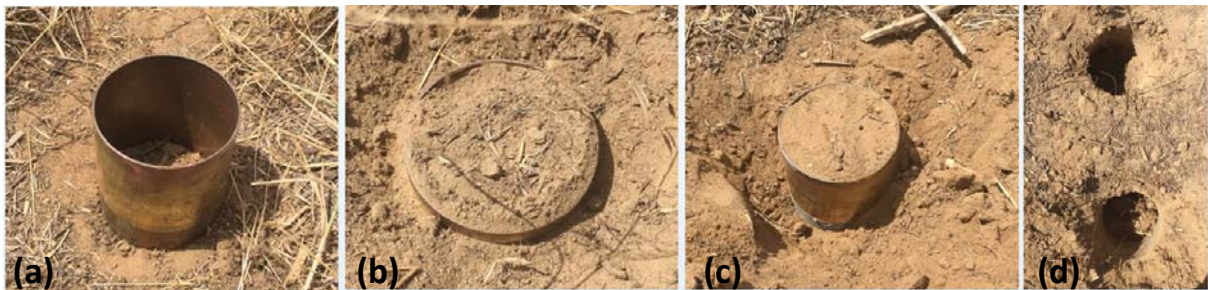
Figure B.3. Drake Farm soil sampling procedure including (a) pressing of brass sampling tube into soil (b) sampling tube advanced completely into the soil (c) removal of soil around brass sampling tube (d) soil after removal of brass sampling tube.
