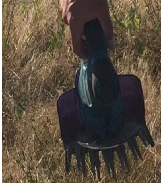
Figure B.2. Electric gardening shears used for removal of surface vegetation before soil sampling.
