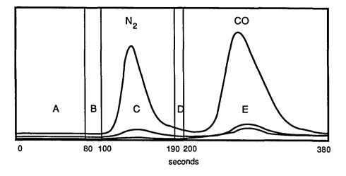
A = initial delay, B = first baseline correction period,  $C = N_2$  integration window, D = second baseline correction period, E = runoff period for CO signal.
