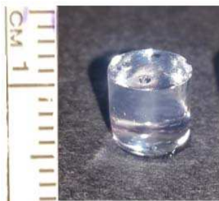
Figure 4. 18 : Thiol-ene hydrogel used in study 5.
