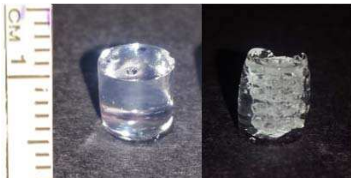
Figure 3. 2 : Left: Thiol-ene hydrogel. Right: PPF scaffold surrounded by thiol-ene hydrogel
