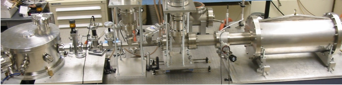
Fig. 3-1: 46.9 nm Ne-like Ar discharge capillary laser and experimental chamber
