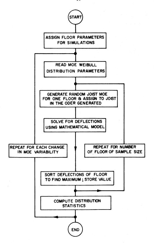
Figure 2.1 SIMULATION PROCESS DIAGRAM
