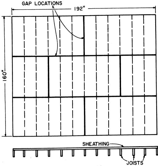
NOMINAL JOIST DIMENSION = 2×8 in. SHEATHING THICKNESS = 0.75 in. SLIP MODULUS = 30,000 lb/in NAIL SPACING = 8 in
