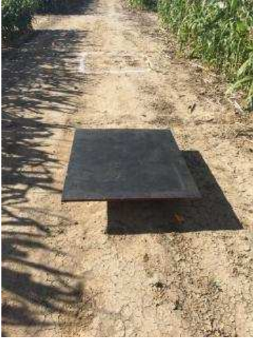
Figure A.1.1.8. Black Reflectance Target. 4' x 4' plywood painted black. The black reflectance target sat at an elevation of 12 inches above the ground.
