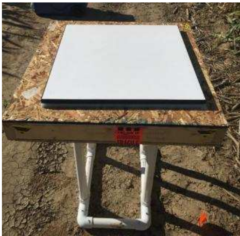
Figure A.1.1.7. Spectralon White Reflectance Target [Spectralon 24 in x 24 in White Target, Labsphere, North Sutton, NH]. The white reflectance target sat at an elevation of 36 inches above ground level.
