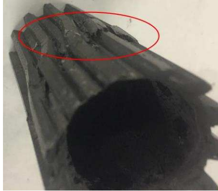
Figure 33: Sample A20 after testing showing fractures in teeth (red)
