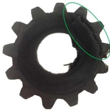
Figure 32: Sample A11 after testing showing separation of teeth from body (green)
