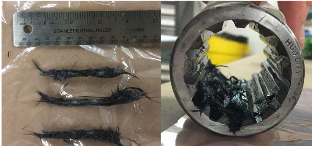
Figure 26: Molding compound charges
