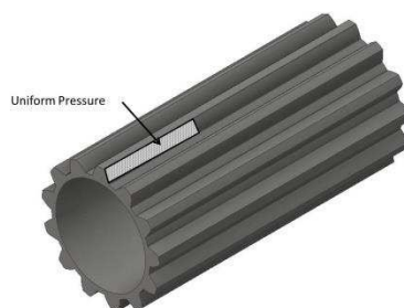
Figure 11: Uniform pressure distribution over spline tooth face
