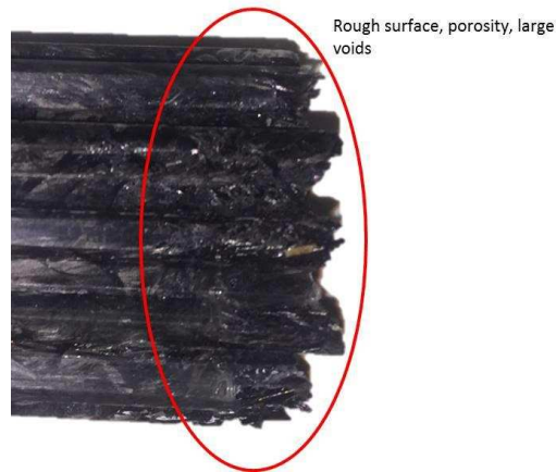
Figure 27: Phase two sample with poor surface finish and voids (red circle)
