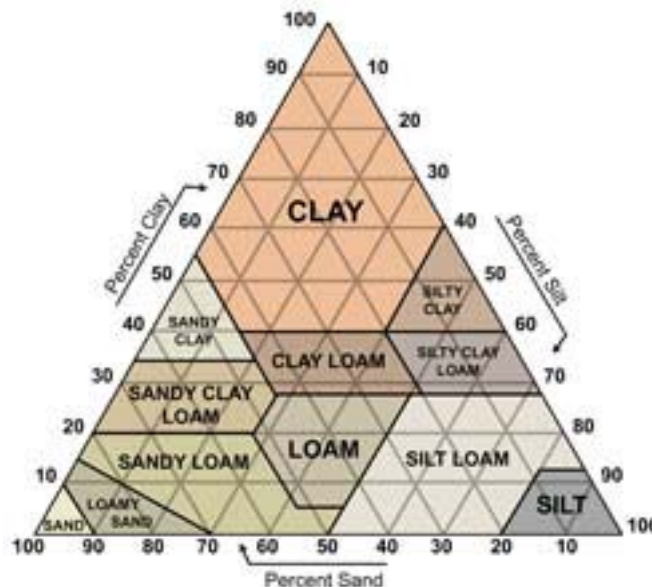
Figure 1. Soil textural classes based on the percentage of sand, silt, and clay.
