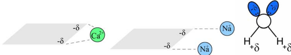
Figure 4. Planner clay lattice with a negative charge distribution and cation influence. Dipole moment of a water molecule.
