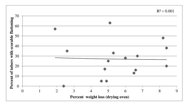
Figure 8. Correlation of moisture loss susceptibility (24 hours at 37°C) with percent of tubers that developed pressure flattening in excess of the USDA No. 1 quality standard after 5 months storage in a commercial storage bin. The R-squared value for the correlation trend line is in the upper right corner of the figure.
