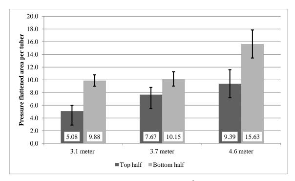
Figure 31. Comparison of averaged pressure flattened area per tuber (cm<sup>2</sup>) by pile height. "Bottom half" treatment is the average of samples that were in the lower half of values when arranged in order of increasing peak load required for 3mm. deformation at harvest. "Top half" treatment is the average of samples in the upper half of values when arranged in order of increasing peak load required for 3mm deformation at harvest.
