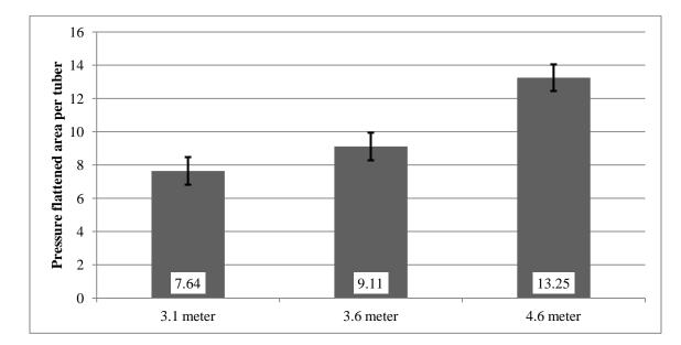
Figure 61. Comparison of pressure flattened area per tuber (cm<sup>2</sup>) based on pile height after 3 months storage duration (averaged across all samples and cultivars).
