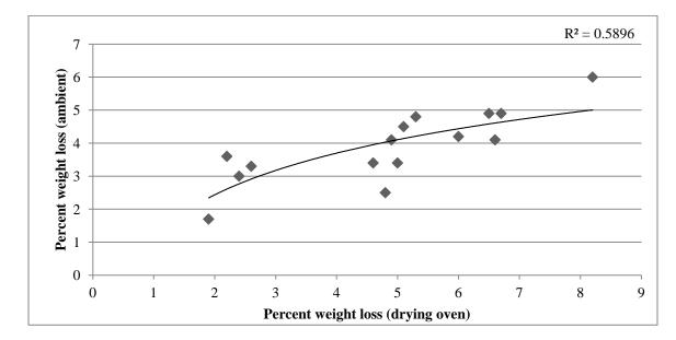
Figure 7. Correlation of percent moisture loss of sets of at harvest samples that were either allowed to lose moisture for 48 hours under ambient conditions (20°C and 45% relative humidity) or for 24 hours in a drying oven at 37°C). The R-squared value for the correlation trend line is in the upper right corner of the figure.
