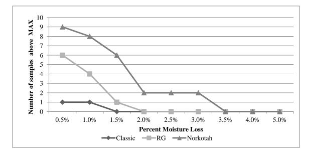
Figure 20. Number of at –harvest samples (out of 20) with a peak load required for 3mm tuber surface deformation that exceeded the 10kg. limit of the texture analyzer as tubers lost moisture following harvest from moist soil (2011 data)
