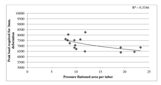
Figure 30. Correlation of 3 month storage duration pressure flattening  $(cm^2)$  for an equivalent 4.6 m. high pile with at-loading peak load for 3mm surface deformation. The R-squared value for the correlation trend line is in the upper right corner of the figure.
