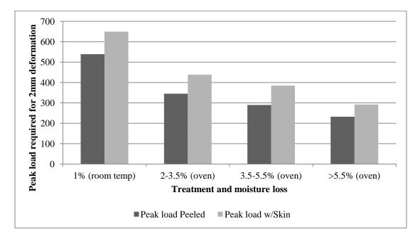
Figure 18. Change in peak load required for 2mm tuber surface deformation of post storage tubers with additional moisture loss treatments. Tubers were tested with skin intact and with skin removed.
