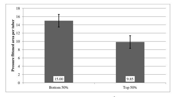
Figure 24. Comparison of averaged pressure flattened area per tuber (cm<sup>2</sup>) across treatments and cultivars after 3 months storage duration for 2011 field experiments. "Bottom half" treatment is the average of samples that were in the lower half of values when arranged in order of increasing peak load required for 3mm. surface deformation at harvest. "Top half" treatment is the average of samples in the upper half of values when arranged for 3mm surface deformation at harvest.
