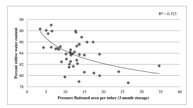
Figure 16. Correlation of at harvest relative water content of tuber tissue cores with the pressure flattened area per tuber  $(cm^2)$  after 3 months storage duration. The R-squared value for the correlation trend line is in the upper right corner of the figure.
