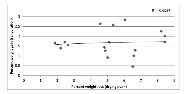
Figure 9. Correlation of percentage of water uptake of samples at harvest (as increase in mass) after immersion in 20°C water for 24 hours compared with percent moisture loss when stored at 37°C for 24 hours. The R-squared value for the correlation trend line is in the upper right corner of the figure.
