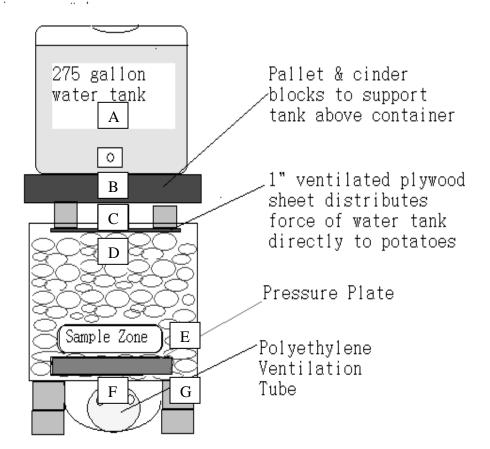
Figure 4. Diagram of the ventilated container design for inducing pressure flattening in storage.
