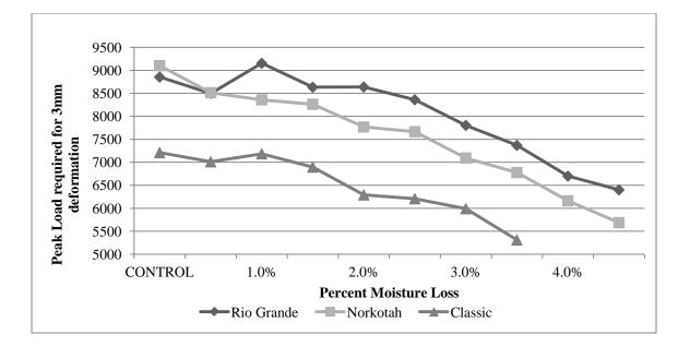
Figure 21. Change in at harvest peak load required for 3mm tuber surface deformation as tubers lost moisture following harvest from moist soil (2012 data).
