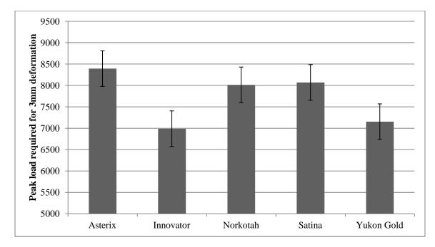
Figure 35. Peak load required for at-harvest 3mm. surface deformation for samples from different cultivars (2012 data)
