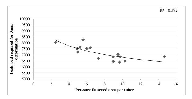
Figure 29. Correlation of 3 month storage duration pressure flattening (cm<sup>2</sup>) for an equivalent 3.1 m. high pile with at-loading peak load for 3mm surface deformation.
