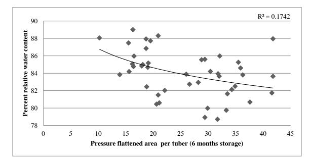
Figure 17. Correlation of at harvest relative water content of tuber tissue cores with the pressure flattened area per tuber  $(cm^2)$  after 6 months storage duration. The R-squared value for the correlation trend line is in the upper right corner of the figure.
