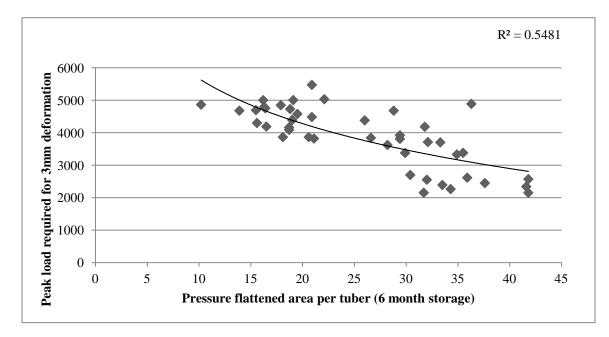
Figure 26. Correlation of at harvest peak load required for 3mm surface deformation with the pressure flattened area per tuber  $(cm^2)$  after 6 months storage duration. The R-squared value for the correlation trend line is in the upper right corner of the figure.
