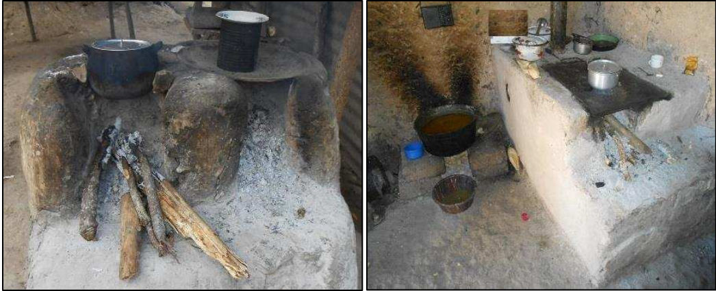
Figure 5.1 Adobe open-fire stove (left), open-fire on floor next to chimney stove (right)
