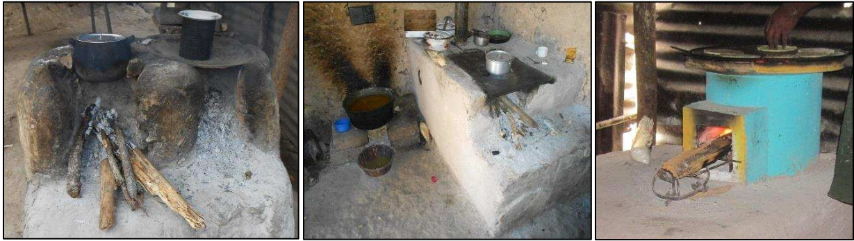
Figure 7.1 Adobe open-fire stove, open-fire (floor) next to chimney stove, Ecocina intervention stove
