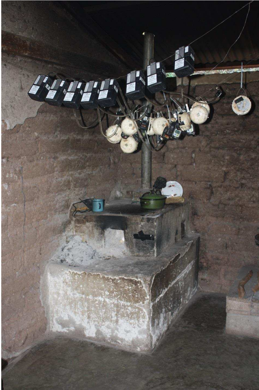
Figure H.1 Photo of instruments placed near a stove during a collocation
