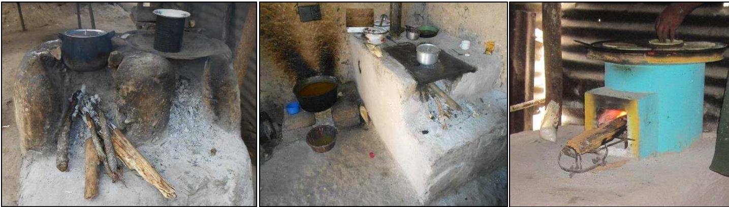
Figure 6.1 Adobe open-fire stove, open-fire (floor) next to chimney stove, Ecocina intervention stove
